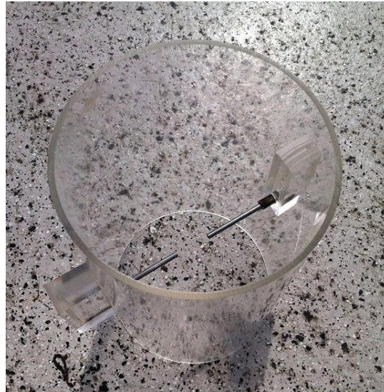
Figure 3.7: Core cylinder of Von Kármán flow facility with nozzles for droplet injection.
