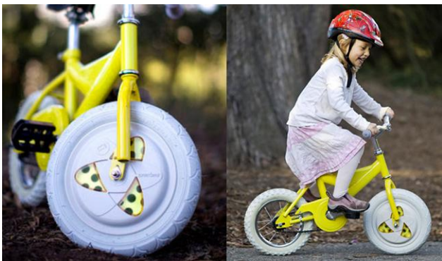
Figure 13. Training wheels have been a necessary evil for many children and their parents. The 'Gyrowheel' Gyroscopic Training Wheel replaces a bike's standard front wheel and features a battery powered spinning disc inside that creates a "gyroscopic precession" force. This force stabilizes the bike and prevents it from wobbling or falling over. Not only will this product make the lives of parents easier, it will provide a more rewarding training process for children and, according to the company, should empower them with better riding techniques.
