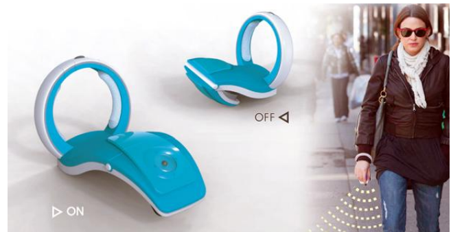
Figure 11 'Supersonic Stick' (by Minhye Kim), is a wrist-worn accessory that can escort the blind. By incorporating sonar technology in a wrist-worn accessory blind people no longer need their blind canes. The 'Supersonic Stick' sends out ultrasonic pulses, and with the spatial information it receives in return, it communicates oncoming obstacles to the wearer in the form of resonant or vibrating messages.
