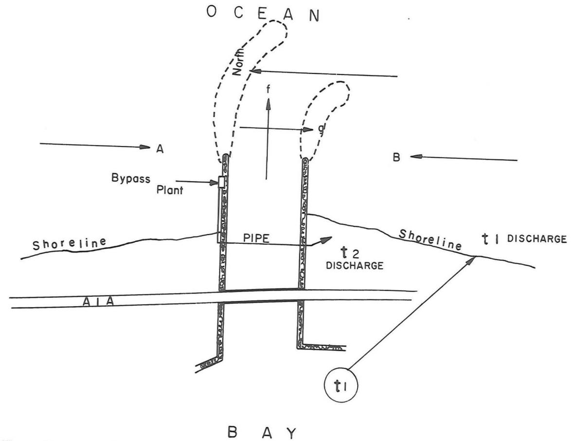
Figure 15. Material Balance at the South Lake Worth Inlet, Florida. Extension of Jetties Indicated by Dotted Lines
