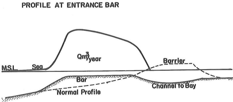
Figure 2. Change of Littoral Drift Pattern caused by Break-through of an Inlet (Bruun and Gerritsen, 1961)
