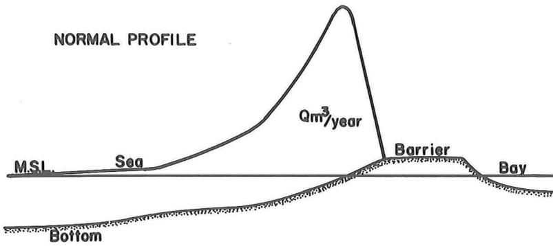
Figure 1. Littoral Drift ( $Mm^3/year$ ) in a Normal Bottom Profile (Bruun and Gerritsen, 1961)
