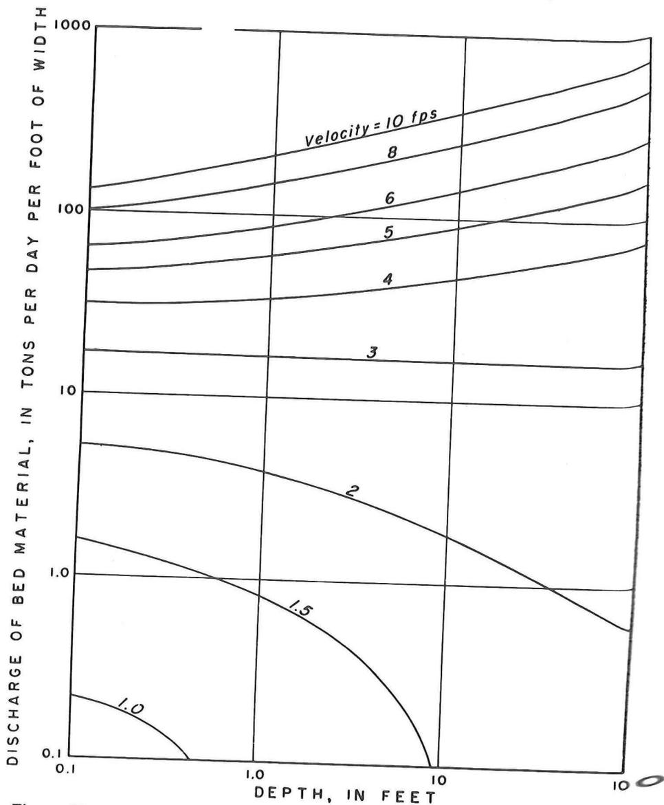
Figure 20. Effect of Depth on the Relationship between Mean Velocity and Empirically Determined Discharges of Bed Material (0.3mm Medium Diameter) at 60° F. B. R. Colby, 1961
