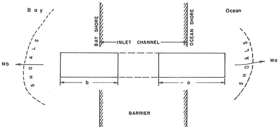
Figure 4. "Rolling Carpet" of Bottom Material in Inlet Channel
