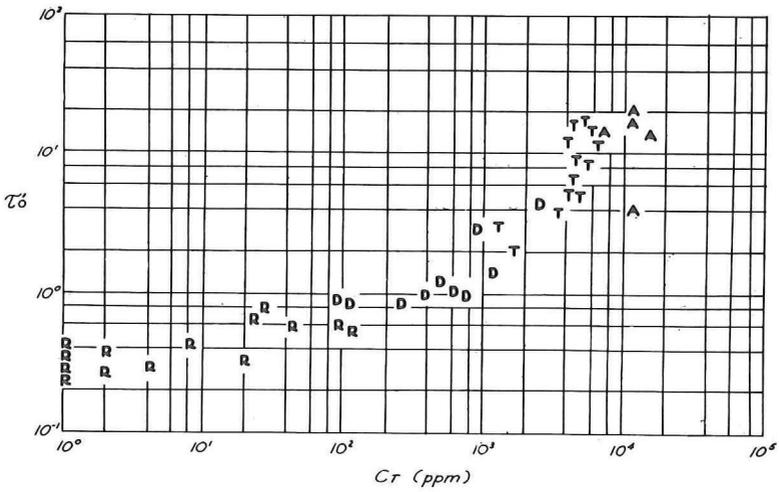
Figure 21. Concentration versus Particle Shear. B. M. Laursen and G. A. Zernial, 1962
