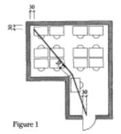
(5) The second stage is escape to a safe place on the ground, often through protected staircases and possibly through (temporarily) safe compartments. The length of a horizontal route within a compartment should be no longer than thirty metres. Communal spaces on a floor level higher than thirteen metres above ground (or five metres for large housing complexes) should have at least one escape route through a protected staircase that gives directly to the ground.
