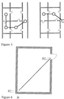
Figure 4 depicts the route in such a space. Note that both the farthest point and the route endpoint by the exit observe a distance of thirty centimetres from building elements. In spaces with two or more exits the space is first subdivided into parts corresponding to the escape field of each exits. Each part is then treated as a space with only one exit. Figure 5 depicts the subdivision of a space with two exits.
