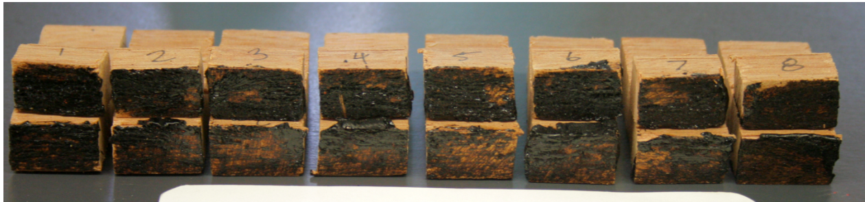
309 310 Figure 7. Bonded surfaces after impact test failures. Even presence of tar on upper and lower adherends indicates failures were 311 cohesive in nature.
