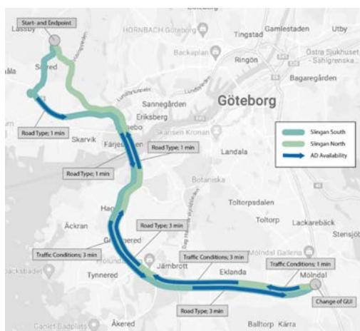
Figure 3.2 Route of a driving session, highlighting stretches of Level 3 unsupervised driving automation availability and exposure time
