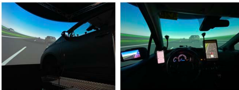
Figure 5.1 Exterior and interior of the DAVSi simulator, with visual UI right of the steering wheel and tablet for the questionnaire left of the steering wheel
