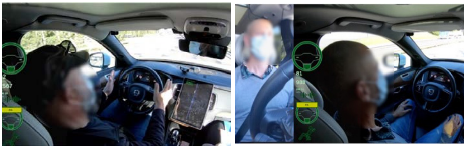
Figure 3.4 Left: Driver testing the steering capability of the Level 2 driving automation; Right: Driver removing hands fully from the steering wheel during Level 2 driving automation
