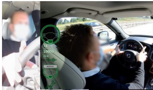
Figure 3.3 The driver attempts to activate Level 3 unsupervised driving automation using the steering wheel buttons in a situation where this mode is not available.
