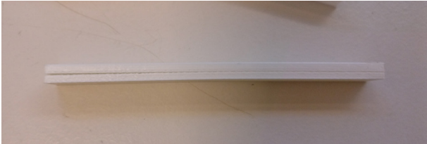
Figure 41 Layer separation present in 3 virgin PLA specimens with perpendicular layer orientation.
