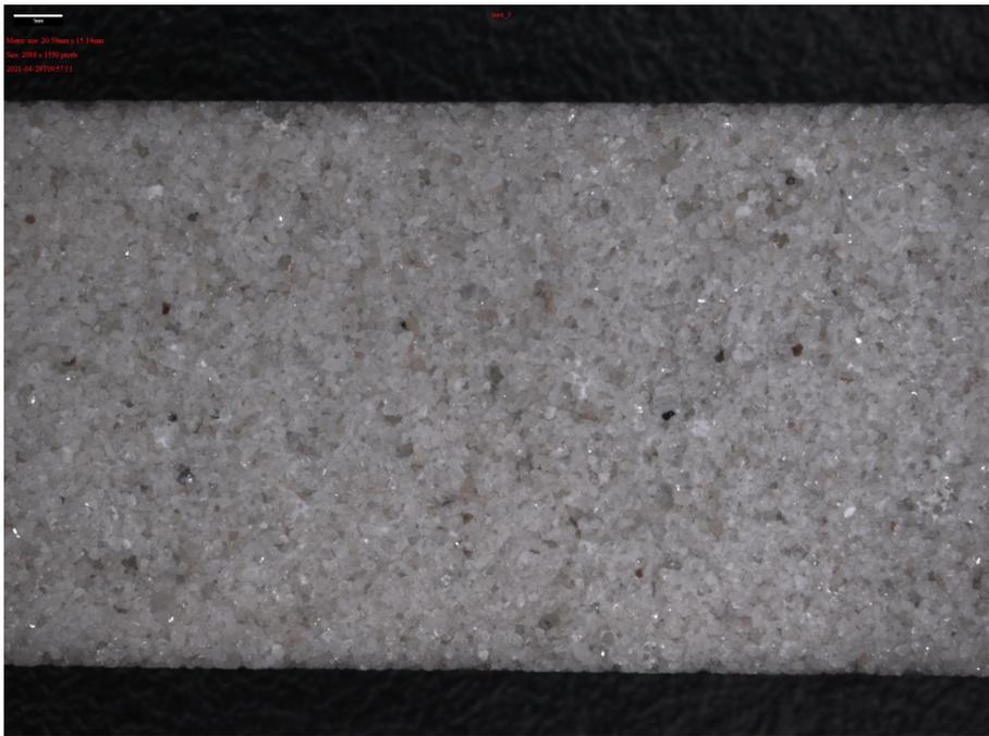
Figure A.4: Bentheimer sandstone used during the initial test with methane and methane-hydrogen mixtures
