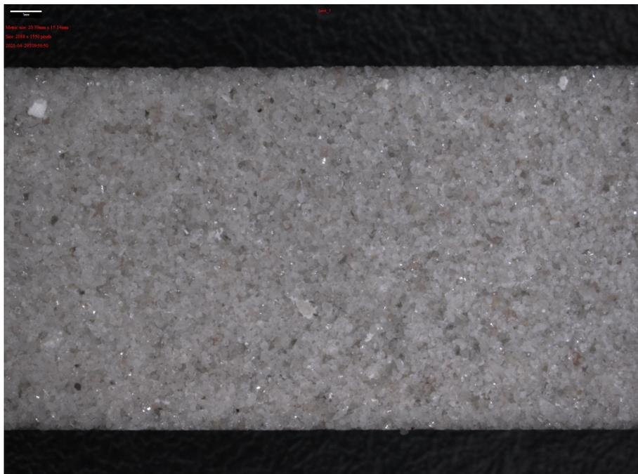
Figure A.1: Bentheimer sandstone used during the repeat test with hydrogen
