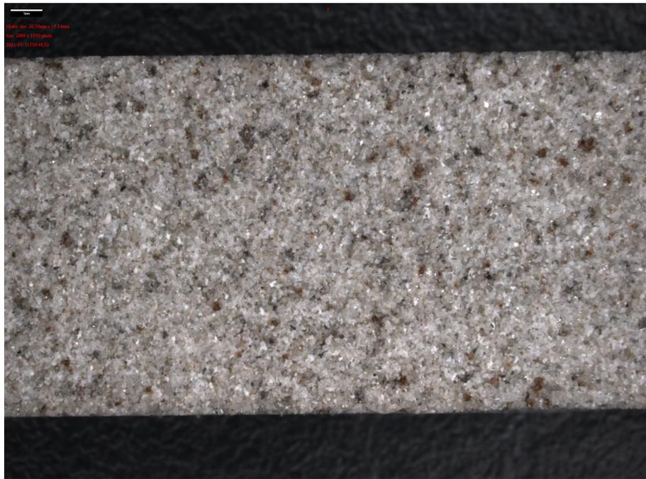
Figure A.2: Berea sandstone used during the initial test with hydrogen
