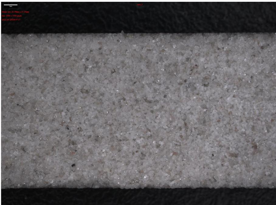
Figure A.5: Bentheimer sandstone used during the repeat test with methane and methane-hydrogen mixtures
