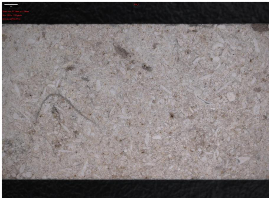
Figure A.3: Edwards White limestone used during the initial test with hydrogen
