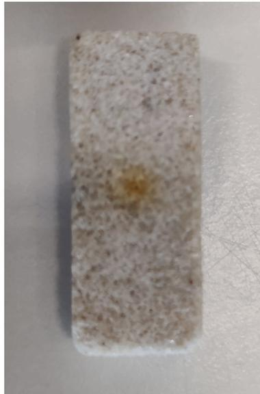
Figure 4.5: Bentheimer sample with a changed color after experimentation
