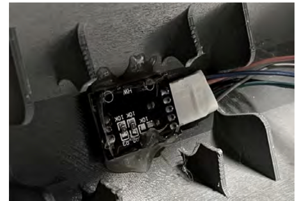
6. Rotary encoder with a button. Pulse circle - 30.
