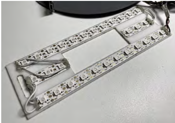
3. Programmable SMD 5050 SK6812 LED strip. 96 LEDs per meter. Luminus flux of LEDs is 208 lm.
