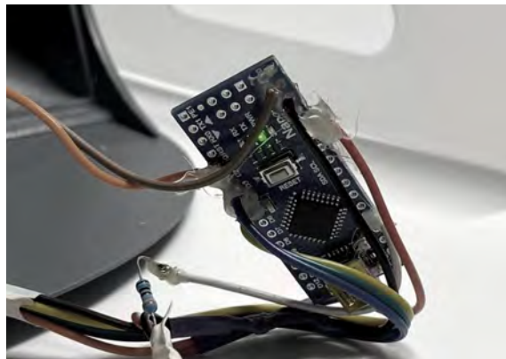
6. Initially, the system was programmed on the Arduino UNO, but then it was moved to the smaller Arduino Nano. For the code, see Appendix X.
