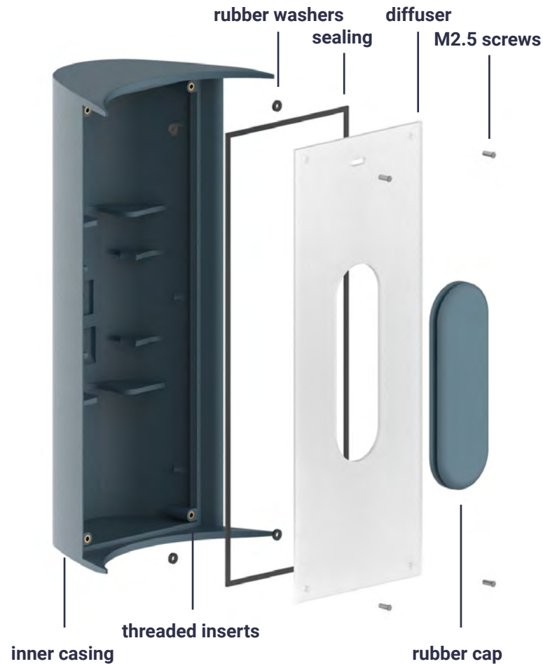
Figure 112: Exploded view of the inner casing
