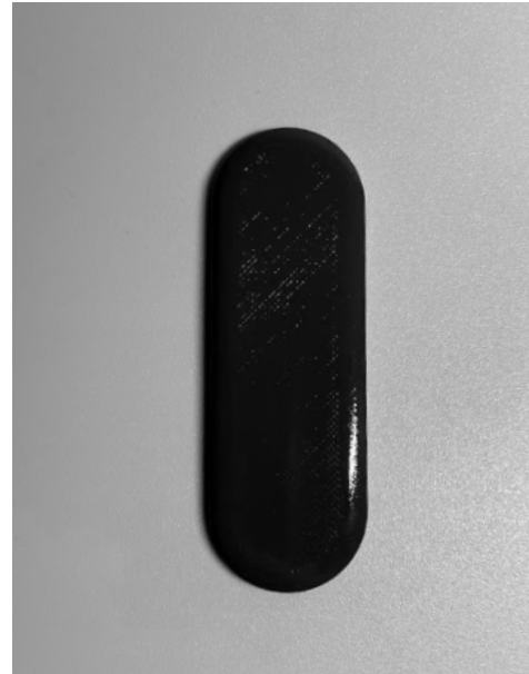
The knob was 3D printed and, just like the chimney, painted with RAL 7031 acrylic spray paint.
