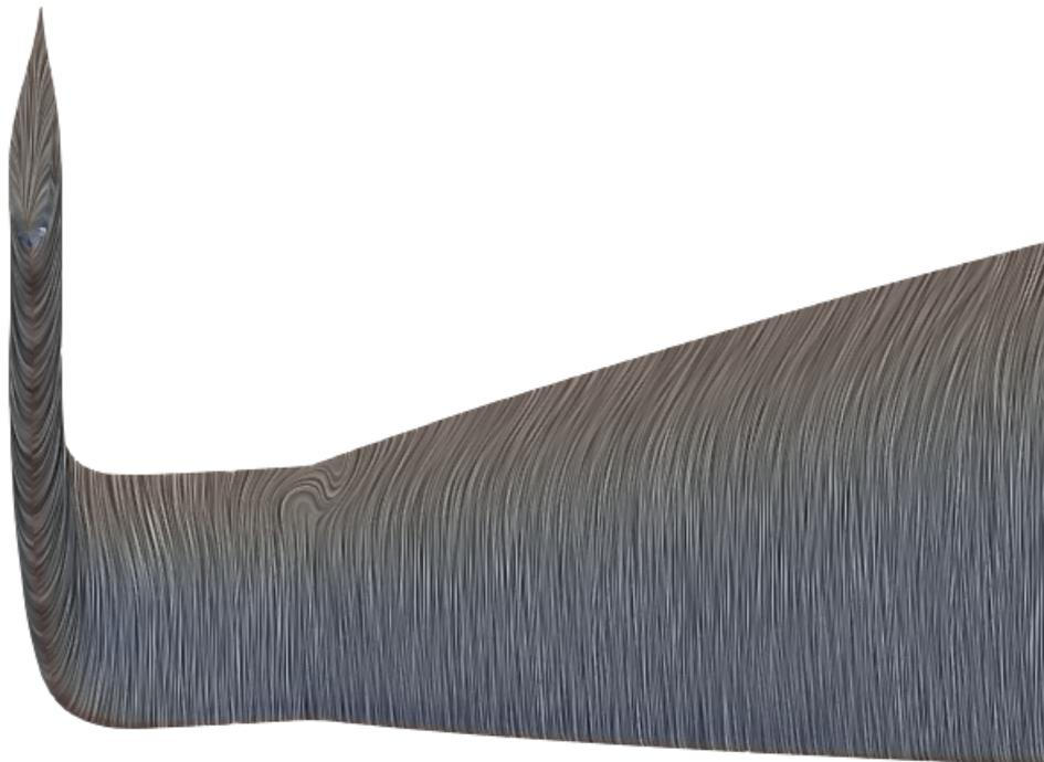
Figure 6.3: Surface LIC of Wall Shear Stress at the Winglet
