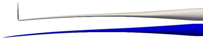
Figure 6.5: Winglet Configuration 2 Geometry
