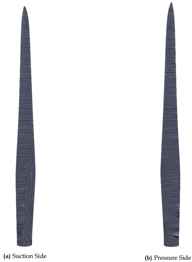
Figure 5.4: Line Integral Convolution of Wall Shear Stress showing massively separated flow at the root section of the blade
