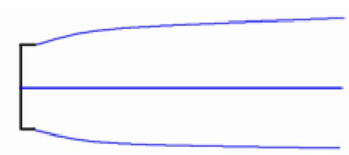
Figure 2.6: The Actuator Cap Model with the actuator cap shown in black and the trailing vortices shown in blue (Gaunaa and Johansen [2007])
