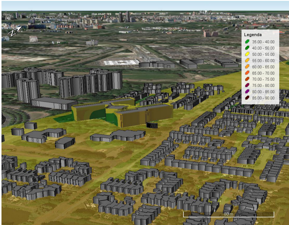
Figure 30: A vertical and horizontal noise contour grid imported into Google Earth Pro .
