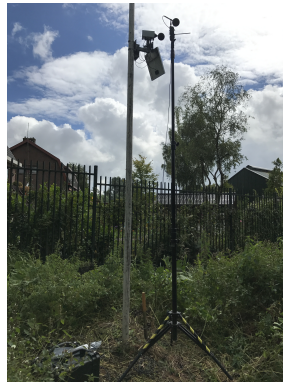
Figure 12: Both systems next to each other at position B, left is Munisense sound level meter and right the MeTrao sound level meter.
