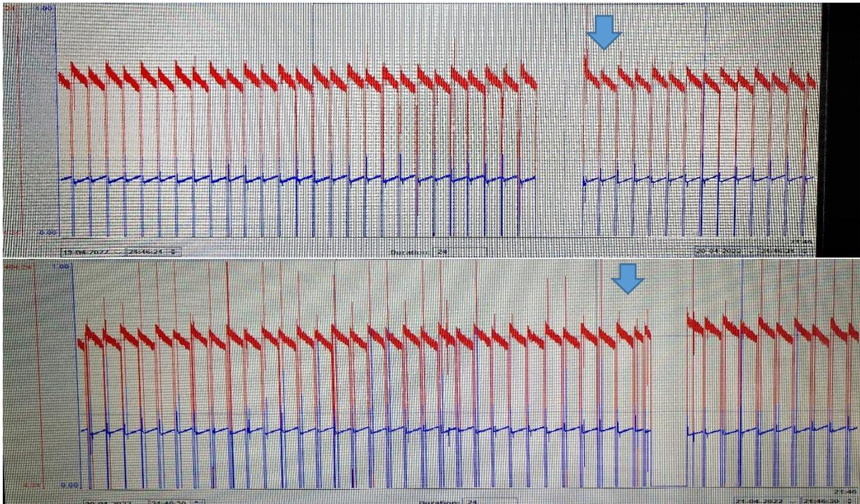
Figure 30 Duplicate experiment 5 fouling (Fe 1.2 mg/l, PAC 15 mg/l). Top: start experiment at blue arrow, before that reference. Gap is due to stop influent water. Bottom: continuation experiment 5, stop at blue arrow. Gap: CEB. Blue is TMP, red is permeability. Scale TMP 0-1 bar, scale permeability 4.24-404.24 l/h/m<sup>2</sup>/bar
