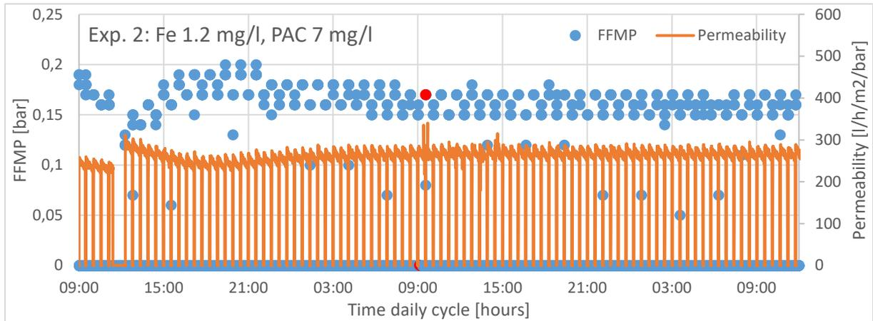
Figure 13 FFMP of UF with dosing of coagulant and PAC. Gap at 11:30 is CEB. Reference up to red dot, red dot is start PAC dosing of experiment 2. (March)
