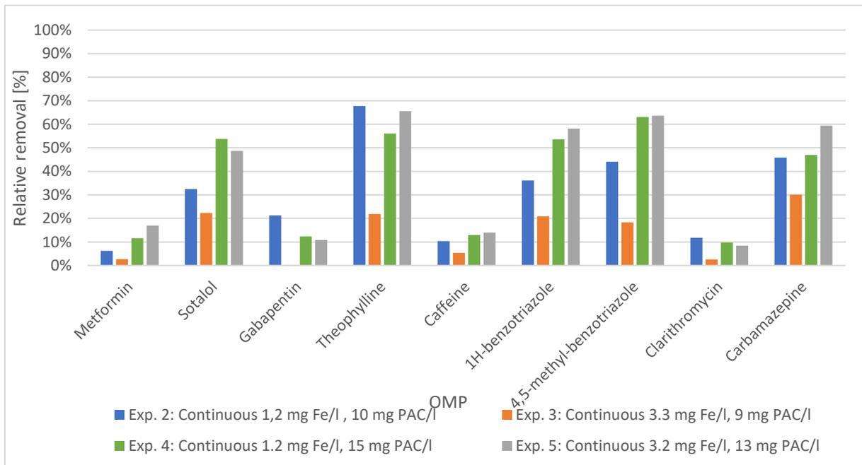
Figure 20 Removal OMP with high and low coagulant doses with inline dosing of PAC and coagulant in UF (n=4). Standard deviations included in Appendix C.3
