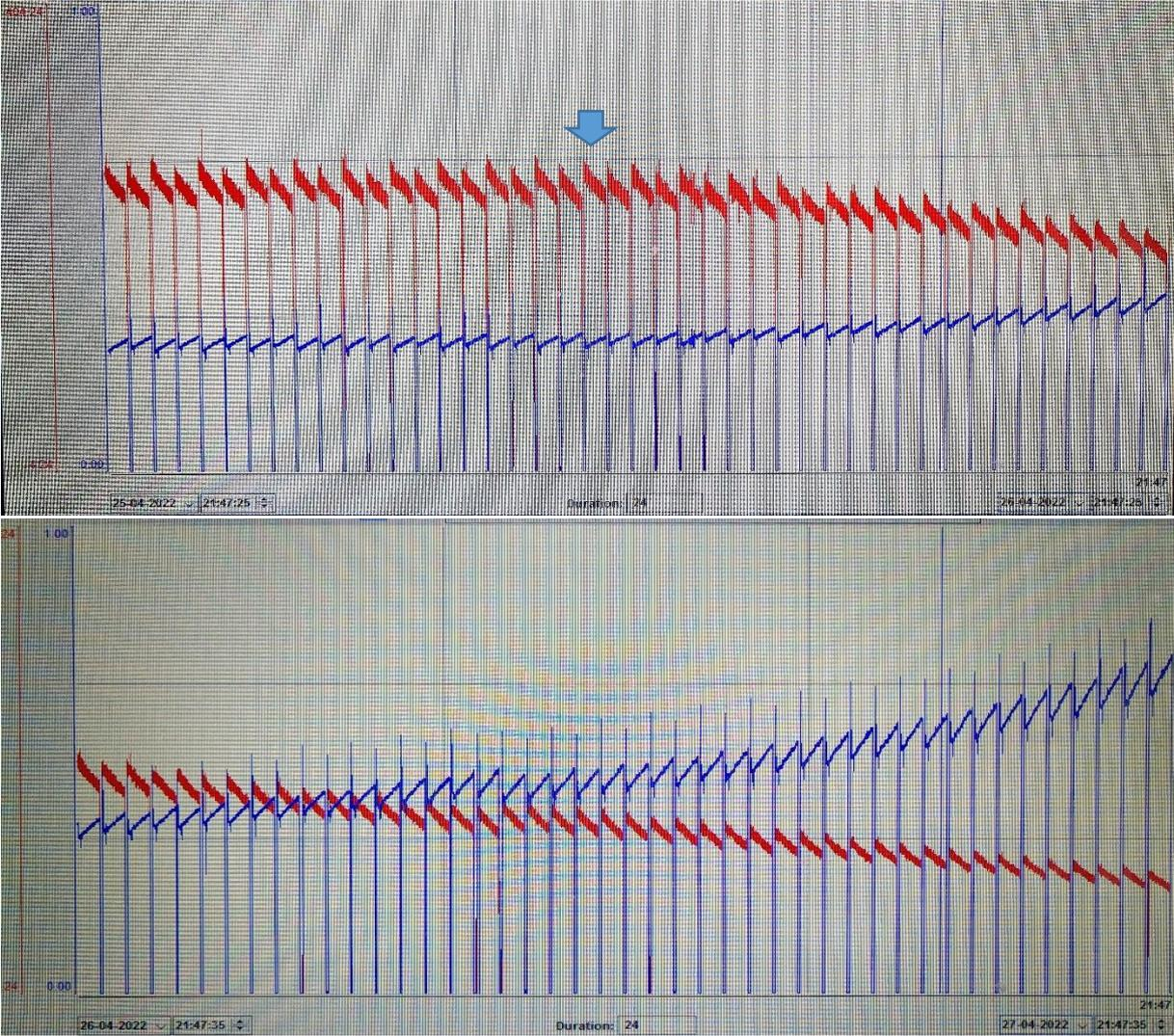
Figure 31 Duplicate experiment 1 fouling (no dosing). Top: start experiment at blue arrow, before that reference (1.2 mg/l) Bottom: continuation experiment 1. Blue is TMP, red is permeability. Scale TMP 0-1 bar, scale permeability 4.24-404.24 l/h/m2/bar
