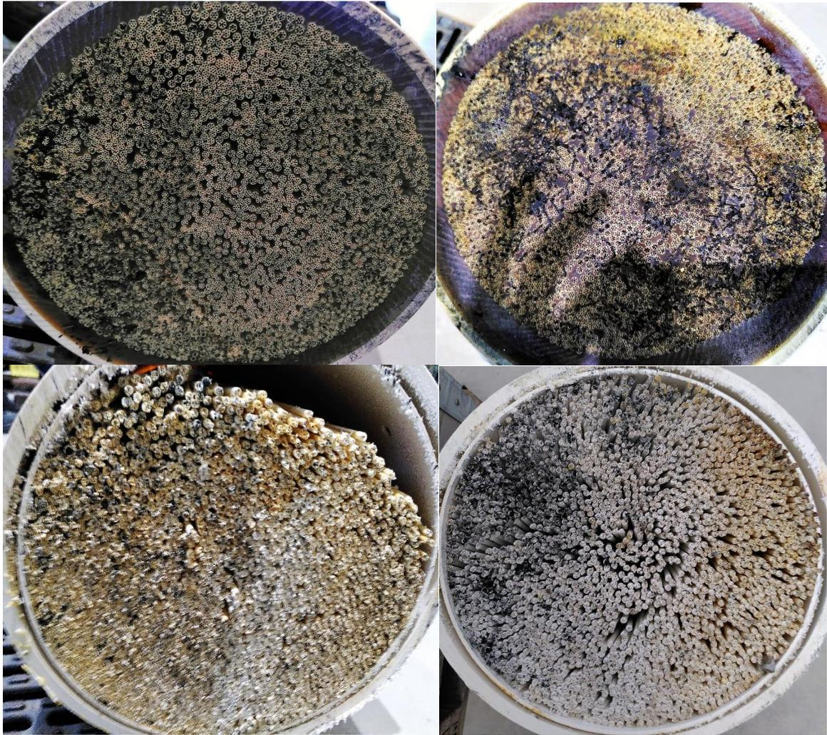
Figure 16 Inside of the membrane after seven months of use with coagulant and PAC. Clockwise starting left top: Bottom, top, bottom half cross-section (wet), top half cross-section (dried).
