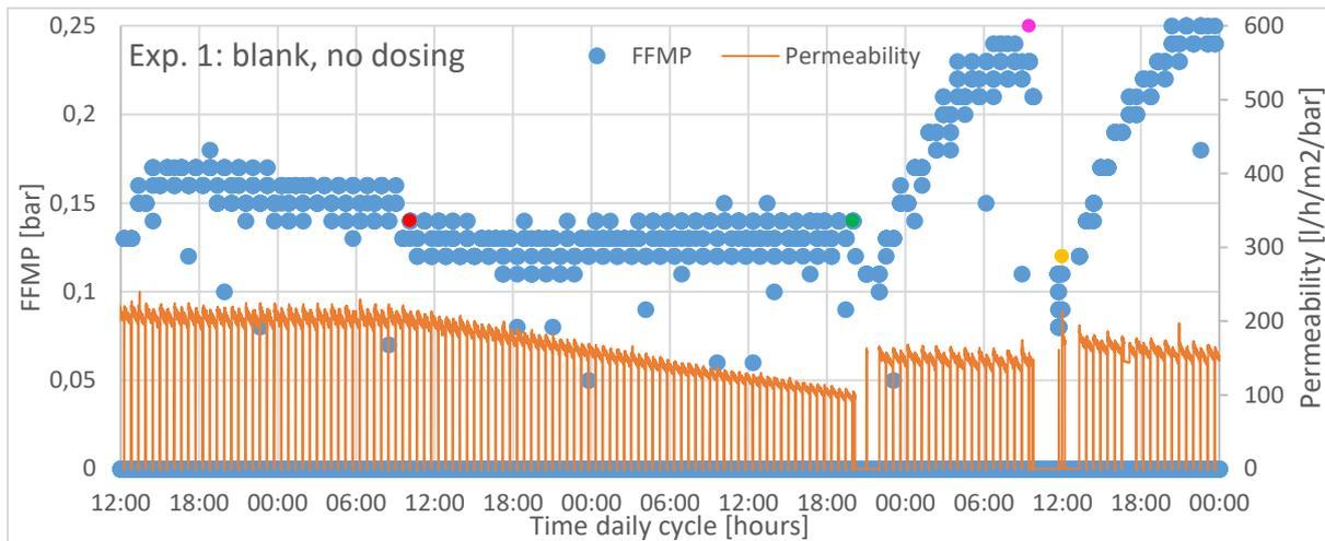
Figure 12 FFMP of experiment 1, UF with blank filtration, no dosing. Reference (up to red dot) 1.2 mg Fe/l, red dot is start PAC dosing, Green acid CEB, Pink and Yellow CEB chlorine. (May)
