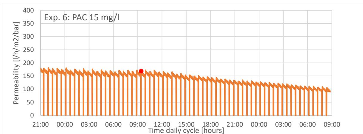
Figure 6 Permeability experiment 6. Reference mode 1.2 mg Fe/l, start experiment 6 at red dot, Pac dosing 15 mg/l
