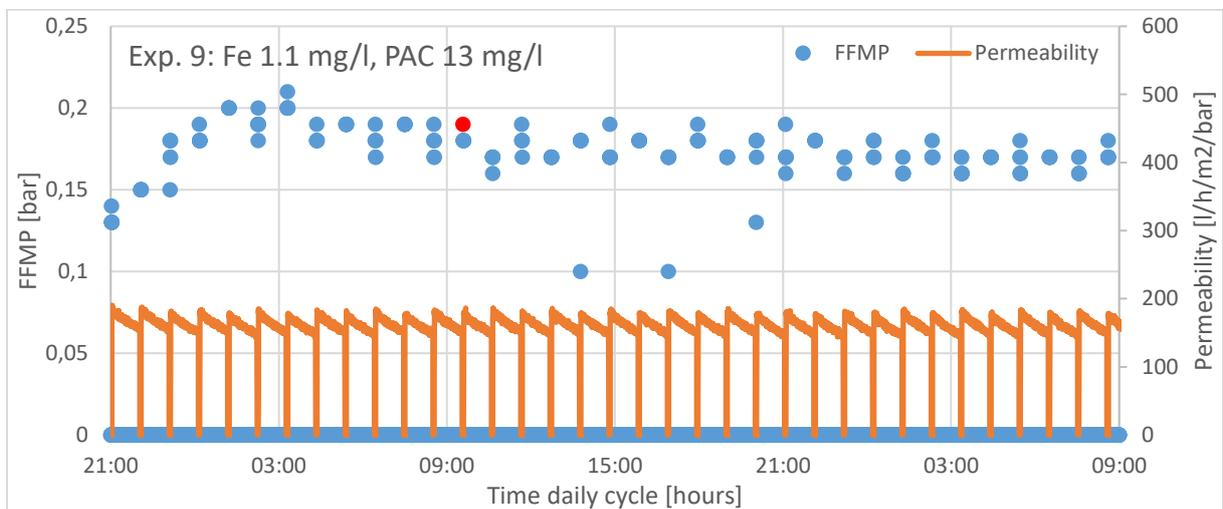
Figure 14 FFMP of experiment 9 UF with dosing of 1.1 mg Fe/l and 13 mg PAC/l with a filtration time of 60 min. Reference (up to red dot) 1.1 mg Fe/l, red dot is start PAC dosing. (May)
