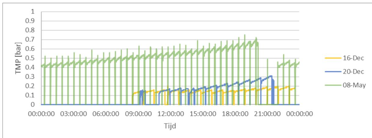
Figure 36. 16 and 20 December filtration time 60 minutes with no addition of coagulant or adsorbant. 8 May filtration time 30 minutes with no addition of PAC or coagulant. Increase in TMP visible
