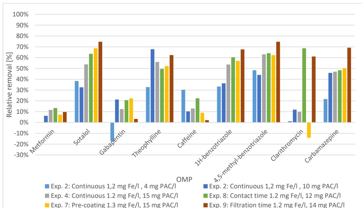
Figure 17 Removal OMP with varying modes of PAC dosing. There are two experiments two due to a large difference in PAC dosing  $n=2$  (4 mg PAC/l) for all others  $n=4$  except for exp. 4 where  $n=6$ , standard deviations included in appendix C.3 .
