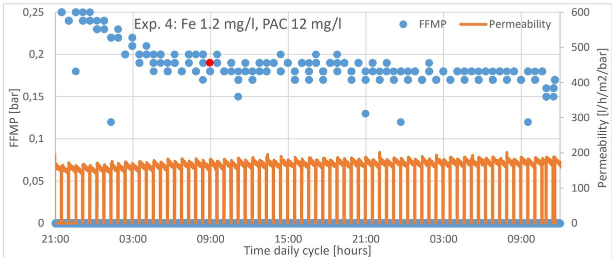
Figure 10 FFMP of experiment 4 UF with dosing of 1.2 mg Fe/l and 12 mg PAC/l. Reference (up to red dot) 1.2 mg Fe/l, red dot is start PAC dosing. (May)
