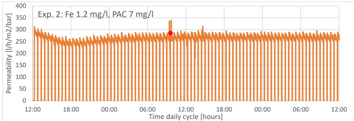
Figure 7 Experiment 2: Permeability with 1.2 mg Fe/l and 7 mg PAC/l. Start at experiment at red dot. Gap around 12:00 at first day is CEB.
