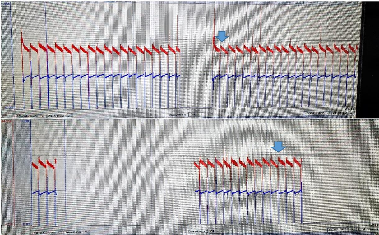
Figure 29 Duplicate experiment 4 fouling (Fe 1.1 mg/l, PAC 7 mg/l). Top: start experiment at blue arrow, before that reference. Gap is due to stop influent water. Bottom: continuation experiment 4, stop at blue arrow. Gap: screen stopped working, UF continued working, no data logged. Blue is TMP, red is permeability. Scale TMP 0-1 bar, scale permeability 4.24-404.24 l/h/m<sup>2</sup>/bar
