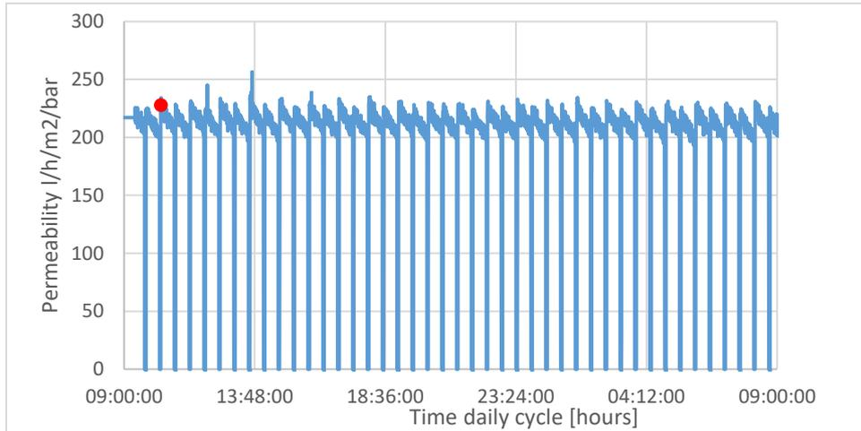
Figure 27 Duplicate experiment 2 fouling (Fe 1.2 mg/l, PAC 6 mg/l). Start experiment at red dot, no reference logged
