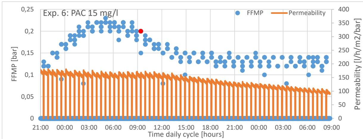
Figure 15 FFMP of experiment 6, UF with dosing of 15 mg/l PAC. Reference up to red dot (Fe 1.2 mg/l), red dot is start PAC dosing and stop iron dosing (May)
