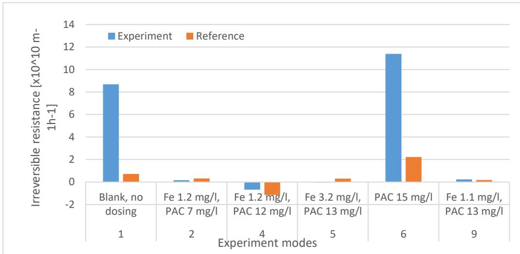
Figure 4 irreversible fouling resistance per hour measured over 24 hours for each experiment mode and 12 hours for each reference mode
