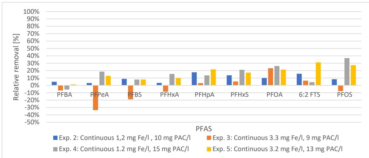
Figure 21 Top: Removal efficiencies PFAS with different coagulant dosing concentrations with inline dosing of PAC and coagulant in UF (n=2). Standard deviations included in Appendix C.3
