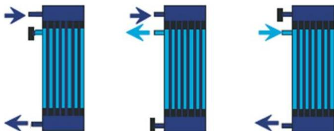
Figure 2 Different filtration modes used for the UF with inline dosing. From left to right: forward flush top, backwash top, filtration top. filtration modes shown for top are the same for bottom except for top being bottom (Logisticon, n.d.)<sup>2</sup>
