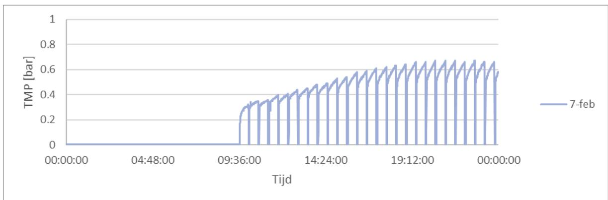
Figure 38 TMP build-up with high turbidity >60 NTU, no addition of coagulant or PAC
