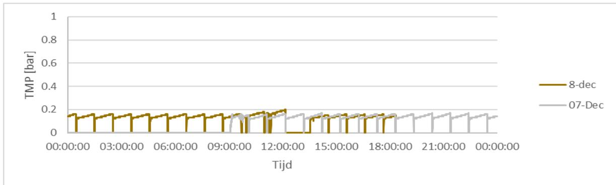
Figure 37 7-8 Dec (until 12:00) December, Filtration time 60 minutes no coagulant no adsorbent, no increase in TMP visible. One day continues at start into the next day.
