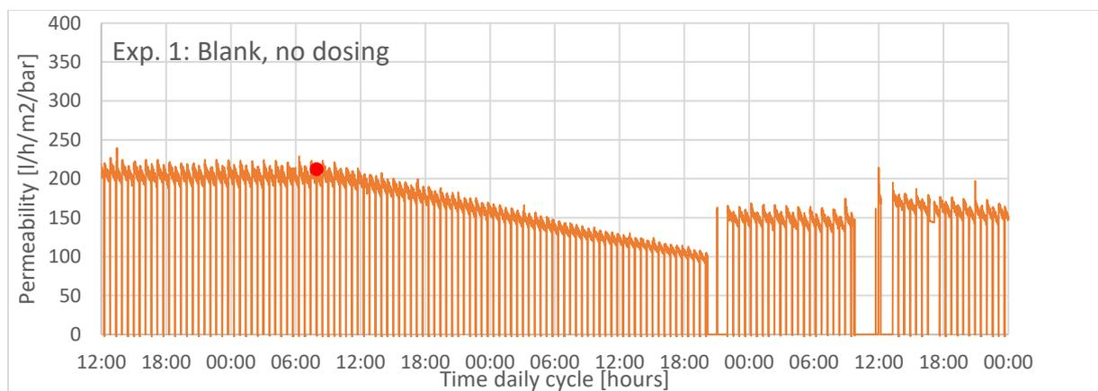
Figure 5 Reference until 10:00, Fe 1.2 mg/l. From 10:00 (red dot) experiment 1: blank filtration no coagulant and no PAC dosing. First gap CEB acid, second two gaps CEB chlorine. (May)
