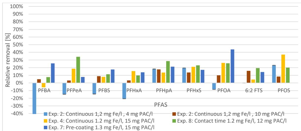
Figure 19 Removal PFAS with varying modes of PAC dosing. There are two experiments two due to a large difference in PAC dosing for these n=1 for all others n=2, standard deviations included in appendix C.3
