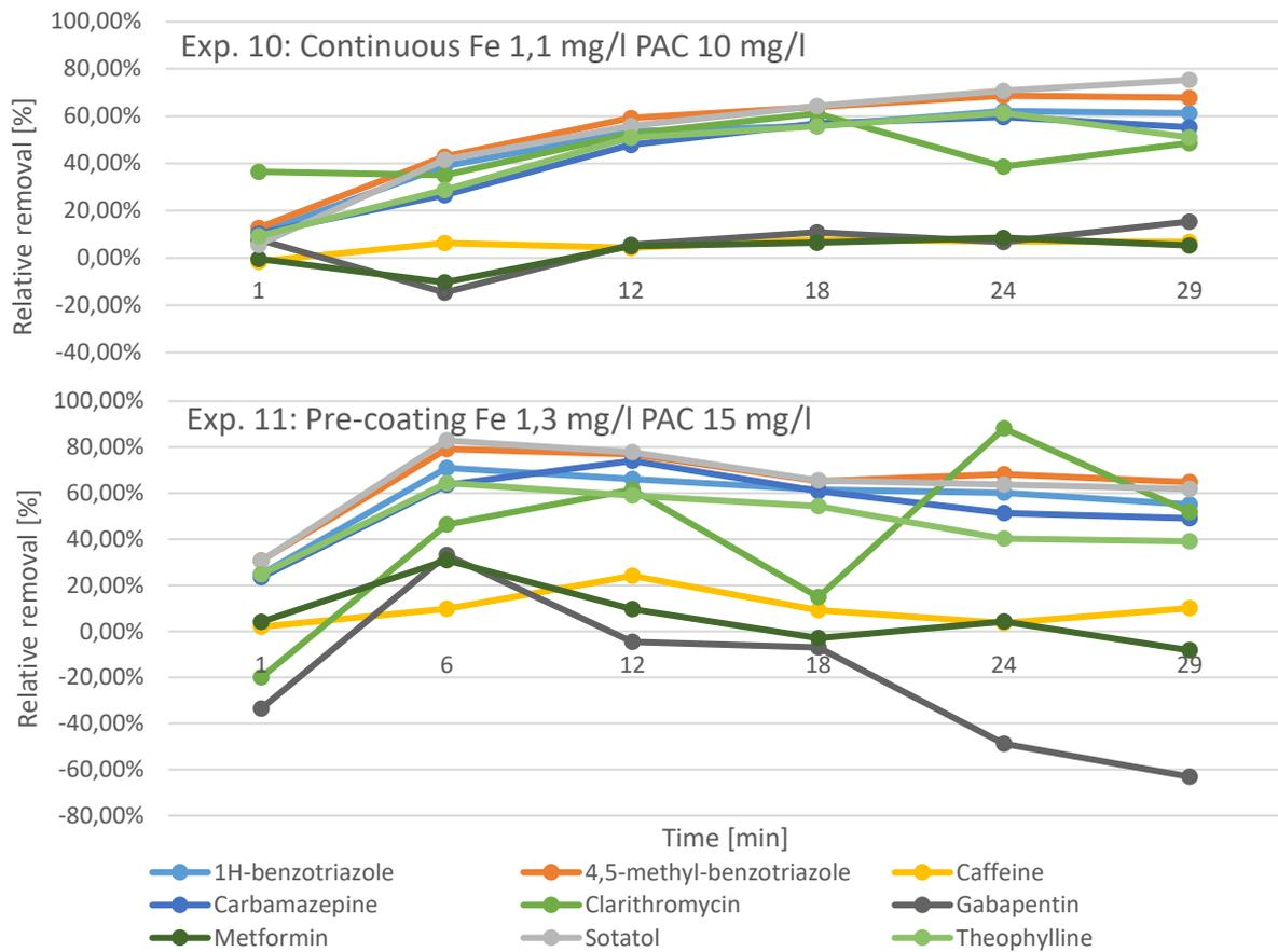
Figure 18 top: Removal efficiency in time with continuous PAC dosing and a filtration time of 30 min (experiment 10), Bottom: PAC pre-coating removal efficiencies in time during filtration cycle of 30 min (experiment 11)
