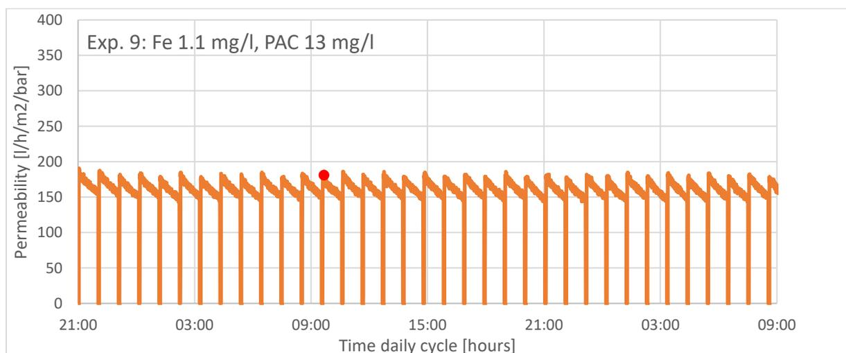
Figure 8 Experiment 9: permeability 21:00 – 09:34 reference (1.1 mg/l), 09:34 (red dot)-09:22 Experiment 9: PAC 13 mg/l and Fe 1.1 mg/l with a filtration time of 60 minutes
