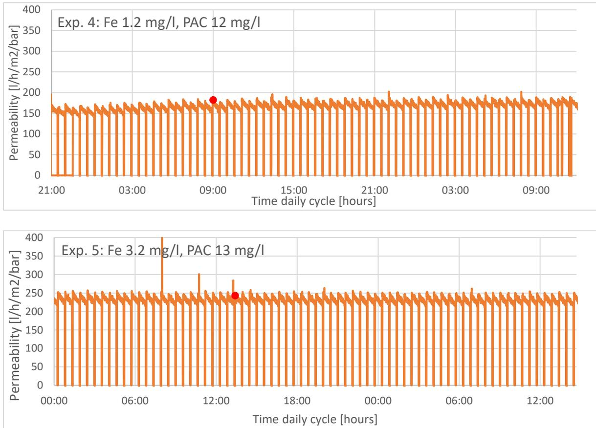
Figure 3 Top: Experiment 4 permeability with 1.2 mg Fe/l and 12 mg PAC/l, reference 1.2 mg Fe/l (May). Bottom: Experiment 5 permeability with coagulant dose of 3.2 mg/l and PAC 13 mg/l, reference 3.2 mg Fe/l
