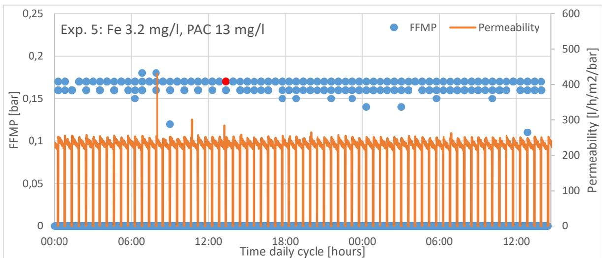
Figure 11 FFMP of UF with dosing of 3.2 mg Fe/l and 13 mg/l PAC. Reference up to red dot, red dot is start PAC dosing experiment 5. (April)
