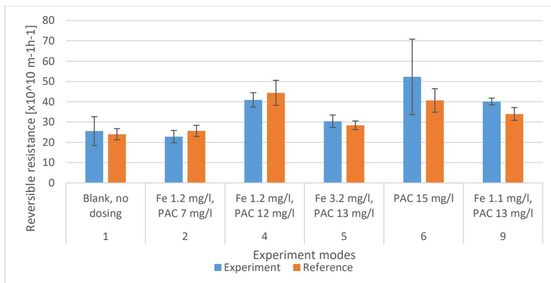
Figure 9 Reversible fouling resistance per hour for top and bottom of each experiment and reference, experiment 9 increase in filtration time 30 to 60 minutes.
