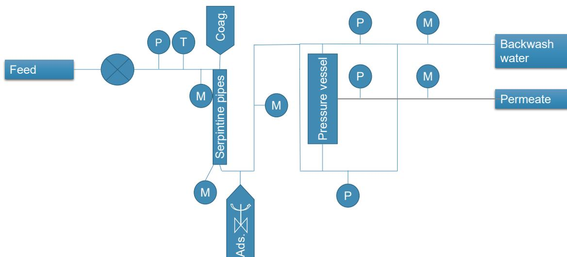
Figure 1 Schematic of the inline UF with the placement of transmitters and sample points
