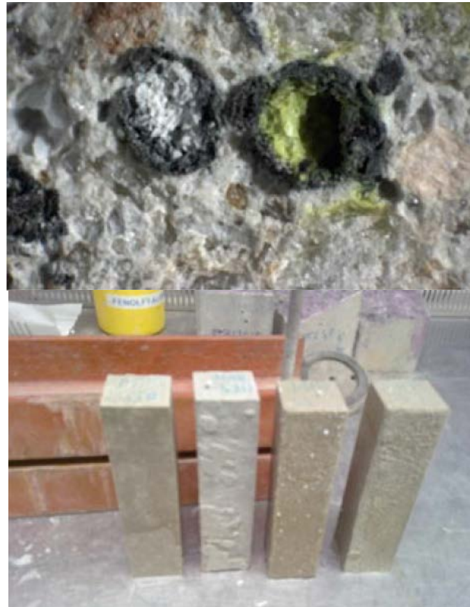
Figure 12: Microscopic view of the concrete— inorganic PCM mixture (left) and test samples of PCM-enhanced concrete (right) (van Haaren 2012)
