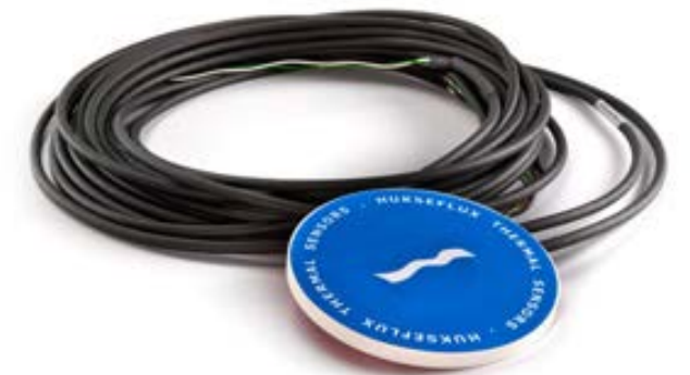
Figure 8.4: The sensor in HFP01 is a thermopile. This thermopile measures the temperature difference across the ceramics-plastic composite body of HFP01. A thermopile is a passive sensor. Reviewed from: http://www.hukseflux.com/product_group/heat-flux-sensors
