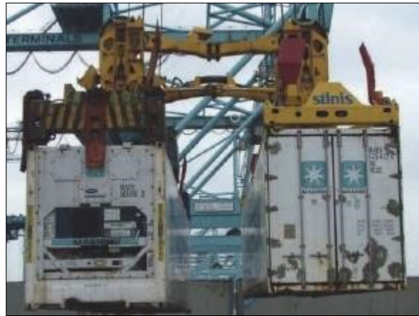
Figure 2.23: Stinis split headblock with two separate spreaders. From [7]
