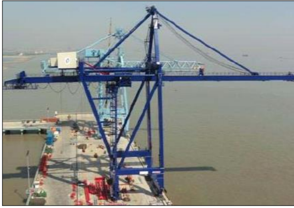
Figure 2.5: Mono girder boom. From [5]
