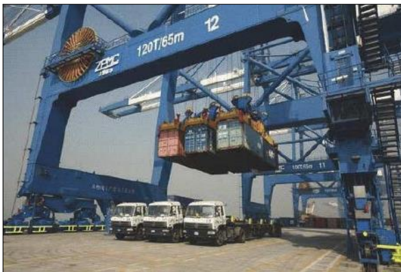
Figure 2.38: Triple lifting. From [7]
