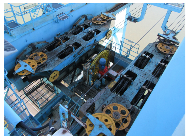
Fig. 11: Trolley with continuous rope support system
