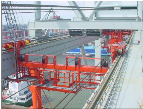
Figure 2.16: Catenary trolley. From [6]
