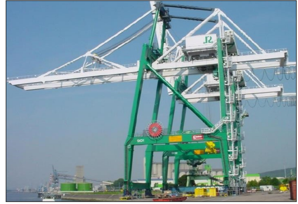
Figure 2.6: Twin girder boom. From [6]
