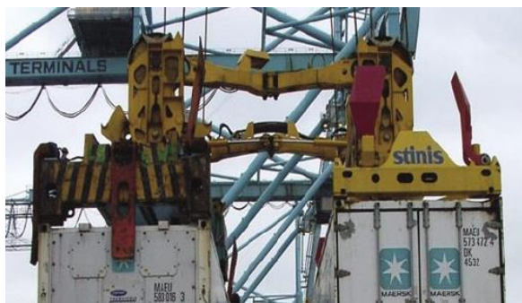
Fig. 1: Single hoist tandem lifting. From [5]
