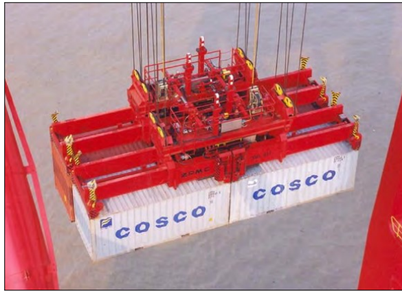
Figure 2.25: Dual hoist tandem lifting. From [20]
