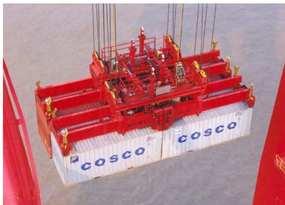
Fig. 2: Dual hoist tandem lifting. From [7]
