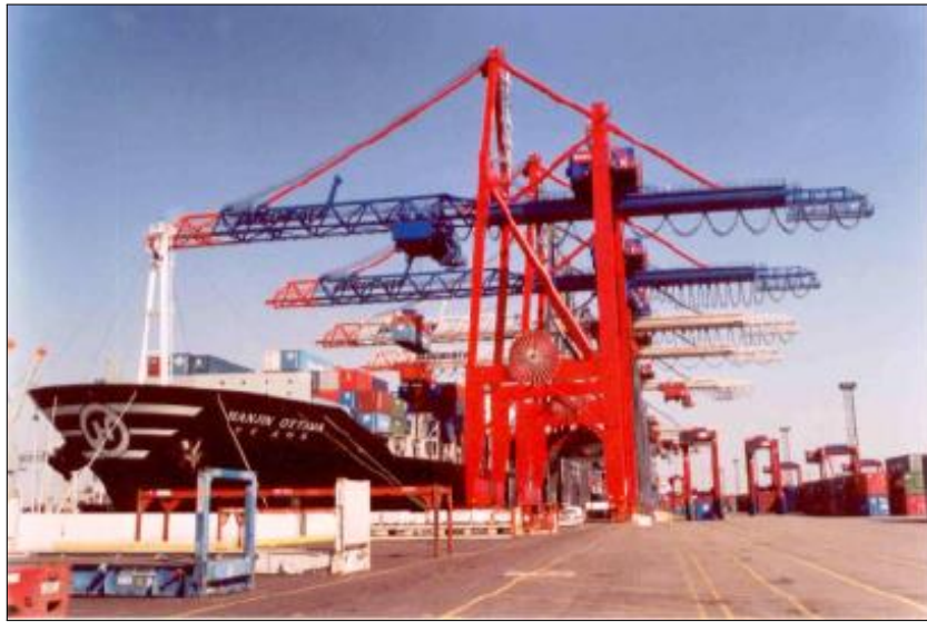
Figure 2.8: Crane with monobox trolley girder and lattice boom. From [6]
