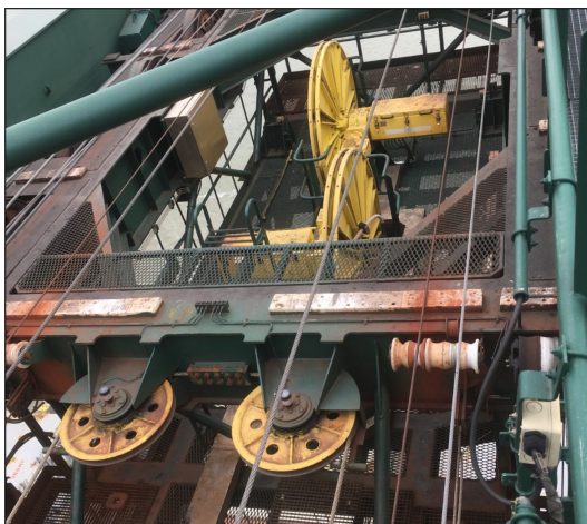
Figure 2.31: Rope towed trolley on a DHT40 crane. From [2]
