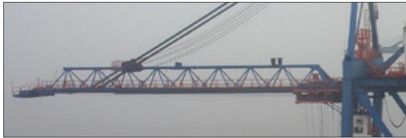
Figure 2.7: Lattice or truss boom. From [4]
