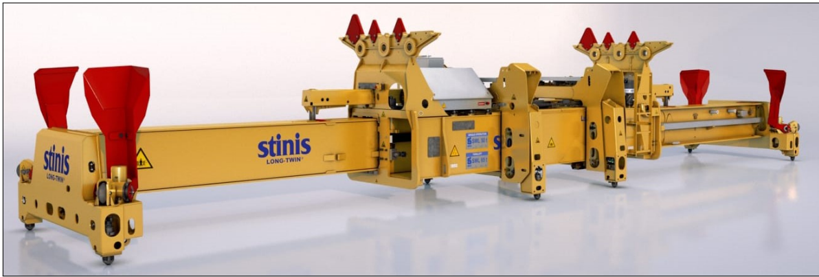
Figure 2.19: Stinis long twin. Load possibilities: 1×20', 1×30', 1×40' 1×45' and 2×20'. From [12]
