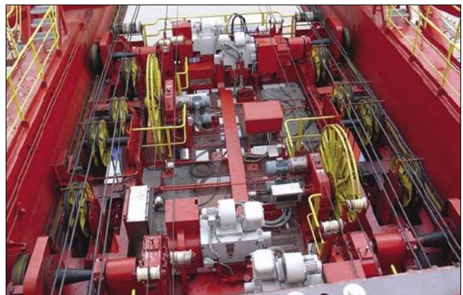
Figure 2.32: Semi rope trolley on a DHT40 crane. From [19]
