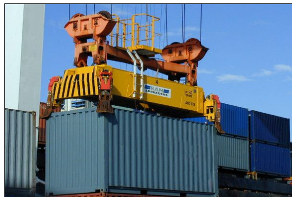
Figure 2.18: RAM 2400 Hydraulic single lift spreader. Load possibilities: 20', 40', 45'. From [11]
