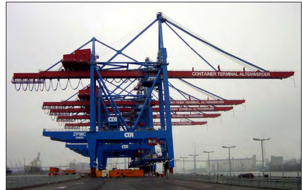
Figure 2.36: Second trolley configuration at Altenwerder container terminal. From [27]
