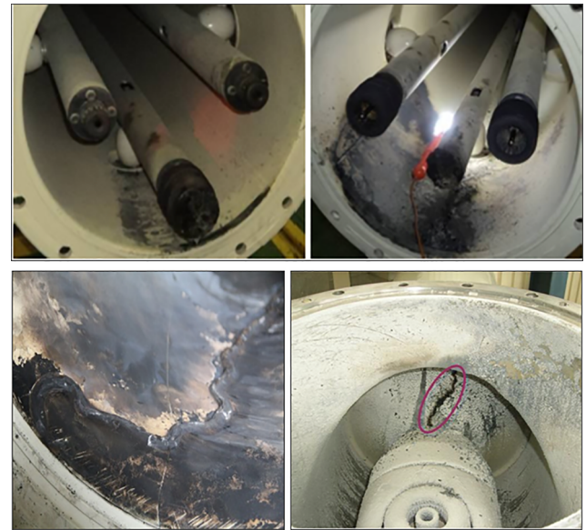
Fig. 2. Failed parts of GIS from the case study. Top: male and female contacts of failed primary joint-conductors. Bottom: insulation breakdown that manifested in flashover of GIS spacer.
