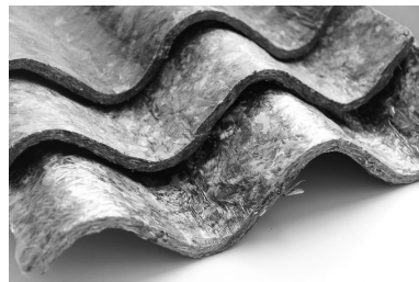
Tuff roof from carton drink packages. Heisel. (n.d.)
