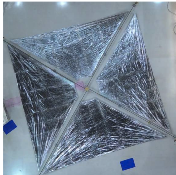
(b) ACS3 prototype unit during the full system ground deployment test of the SBS [118].
