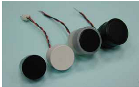
Figure A.1: Air ultrasonic ceramic transducer[1].
