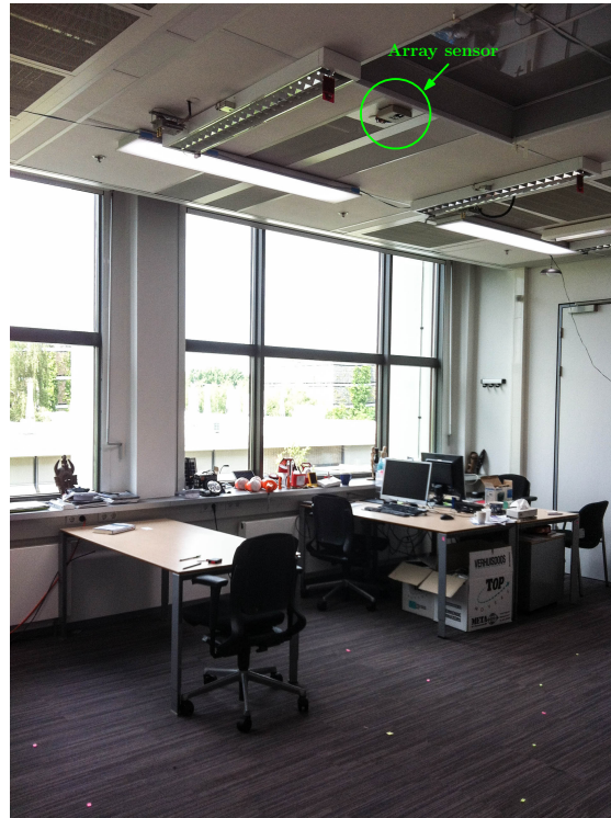
Figure 4.3: Array sensor position in the test office.
