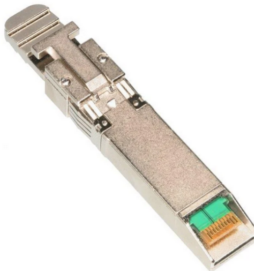
Figure 6.15: SFP loopback adapter. The internal terminals are electronically bridged.
