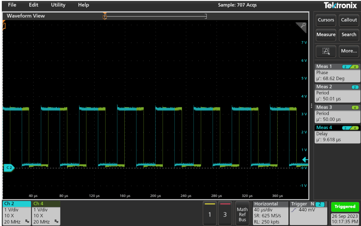
Figure 5.9: DDMTD beat frequencies sampled by a Tektronix Series 2 oscilloscope
