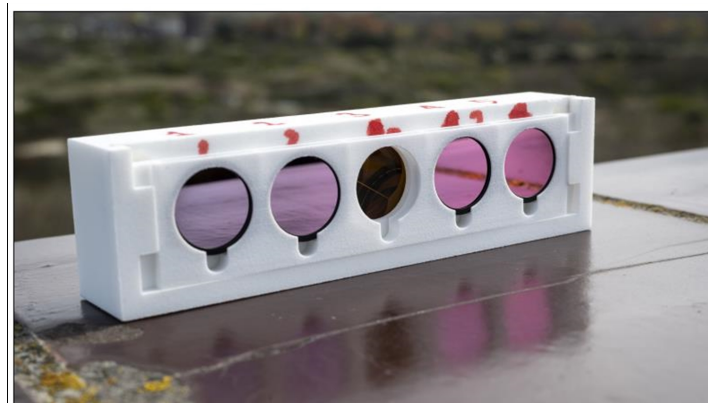
Figure 4.2: Retro-reflector array used in the test setup from TNO 1 .
