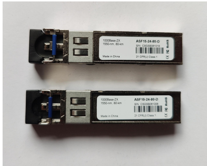
Figure 6.2: ASF-15-24-80-D 1550-nm SFP modules used for in the FPGA
