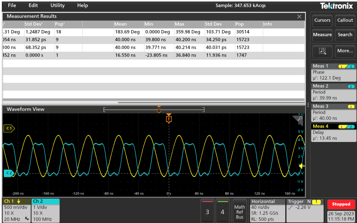
Figure 6.32: Capture of oscilloscope phase measurement between TXUSRCLK2 and RXUSRCLK2
