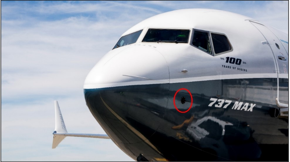
Figure 1.5: Boeing 737 MAX nose with the angle-of-attack (AoA) vane circled; MCAS relied on a single AoA input, a key factor in the 2018–2019 accidents [19].
