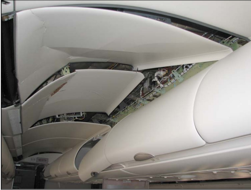
Figure 1.6: Cabin overhead panel damage on Qantas Flight 72 after uncommanded pitch-downs driven by erroneous ADIRU data and flight-control logic (in-flight upset, 7 Oct 2008, 154 km W of Learmonth, WA) [29].
