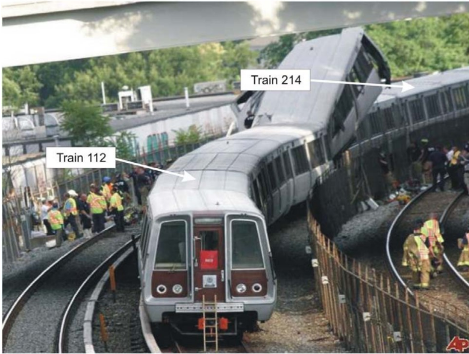
Figure 1.10: Washington Metro Red Line collision near Fort Totten. An automatic train-control/track-circuit occupancy failure commanded a following train into an occupied block, causing a rear-end collision [27].
