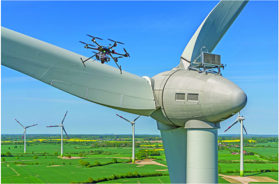
Figure 1.3: Autonomous multirotor inspecting a wind-turbine blade—shifting hazardous, high-altitude maintenance to unmanned systems while requiring robust perception, gust-resilient control, and fail-safe behaviours.
