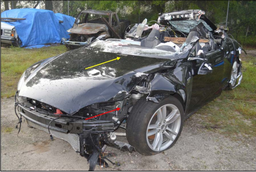
Figure 1.8: Wreckage of the Tesla Model S (Williston, Florida). With Autopilot engaged, the system failed to detect a crossing tractor-trailer; insufficient driver oversight resulted in a fatal underride [24].
