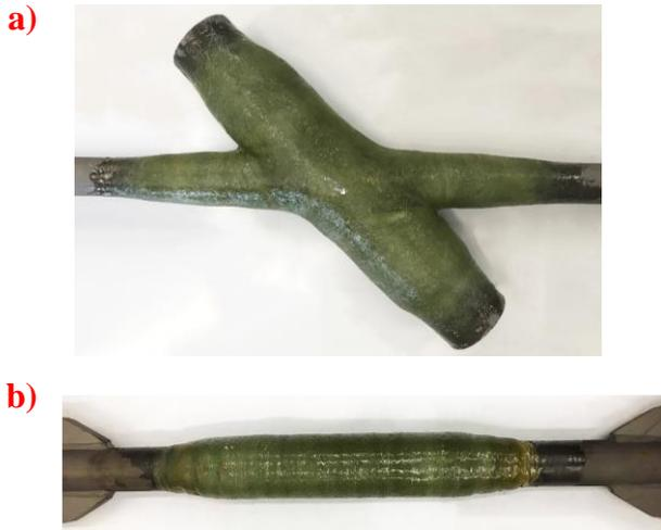
**Figure 3-2 Composite wrapped small-scale a) 45° X-joint with Ø 60 mm braces[15] and b) A-joint with Ø 60 mm steel tubes in lab tests[17].**
