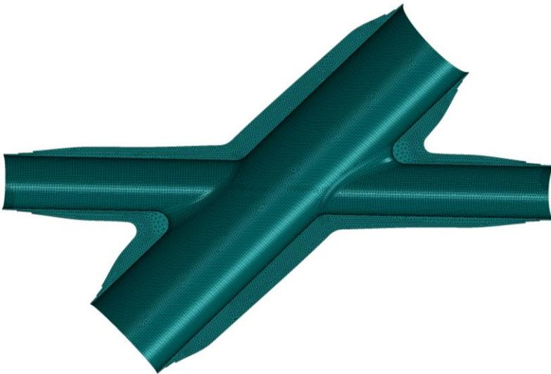
**Figure 5-2 Modelling composite wrap of wrapped composite joints using 3D solid elements (4-node linear tetrahedral elements, C3D4)**
