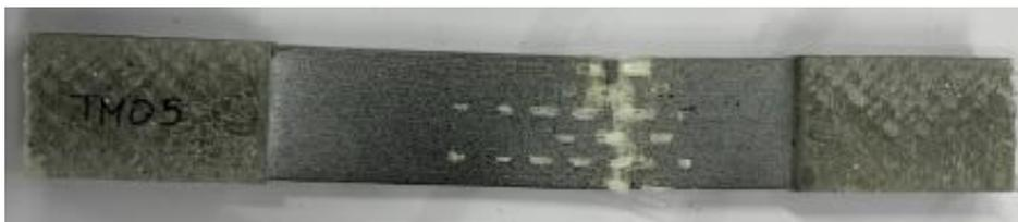
**Figure 4-6 Failure mode of tensile rupture of composite material in tensile coupon tests**
