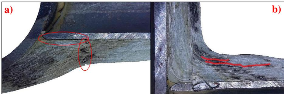
**Figure 3-36** View of cut-plane of small-scale wrapped composite 90° X-joint specimens loaded in bending representing a) debonding on primary bonded interface and fracture of composite wrap on the joint side; b) delamination of composite wrap in the compressive zone
