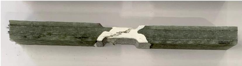
**Figure 4-8 Failure mode of delamination of composite material in compressive coupon test**
