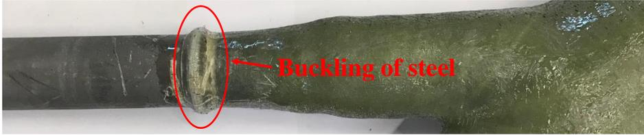
**Figure 3-28 Buckling of brace outside the composite wrap in compressive static test**
