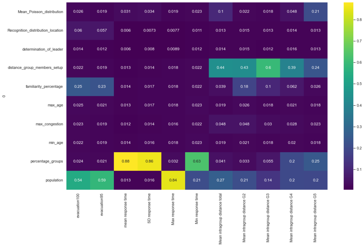
Figure 5.2: Feature scoring for the uncertainties. A higher number indicates a greater influence on the Key performance indicator.
