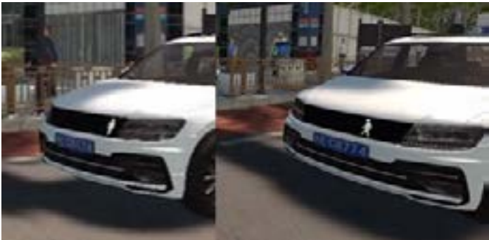
Figure 47 The eHMI with the symbol's appearance adjusting based on the participant's position and pedestrian activity, displaying either a stationary (left) or animated walking pedestrian (right).
