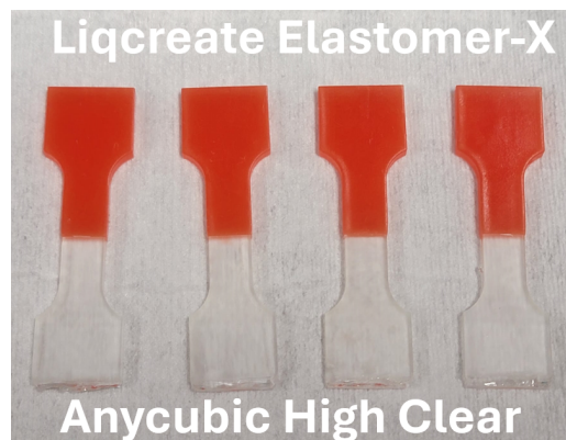
Figure 6.12: MMAM dog bones, created in Anycubic High Clear and dyed Liqcreate Elastomer-X.
