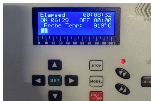
Figure 6.9: Temperature of IPA bath during ultrasonic cleaning is observed to be 19 degrees Celsius
