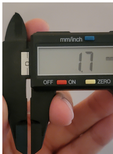
Figure 6.5: Calipers were used to validate if the printed object has the correct dimension, as edited in the UVTools software.
