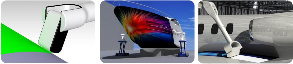
FIGURE 14: THE PRINTING HEAD WILL BE ABLE TO APPLY (FUNCTIONAL) COATINGS ON WIND TURBINES, SHIPS AND AIRCRAFT (GROOT, 2018)
