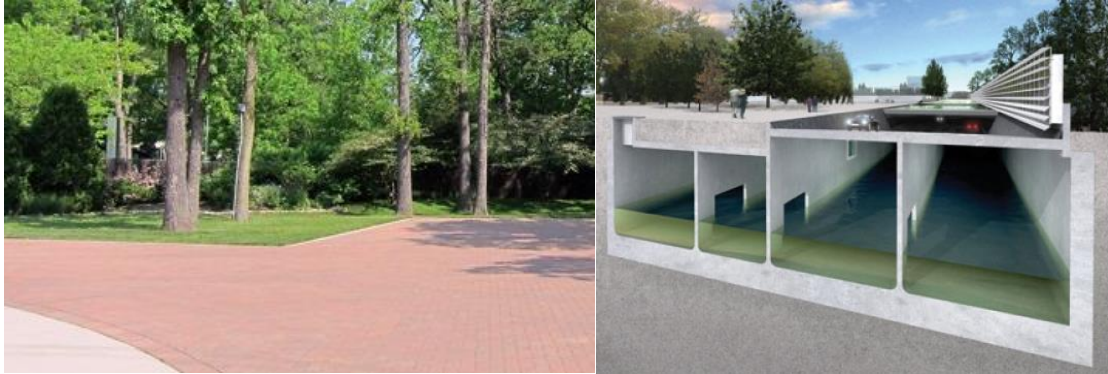
Figure 60 Left: Parking lot on top of storage tank, Illinois (Source: la foundation) and right: storage beneath parking garage, Rotterdam (source: Nooijer, 2011)
