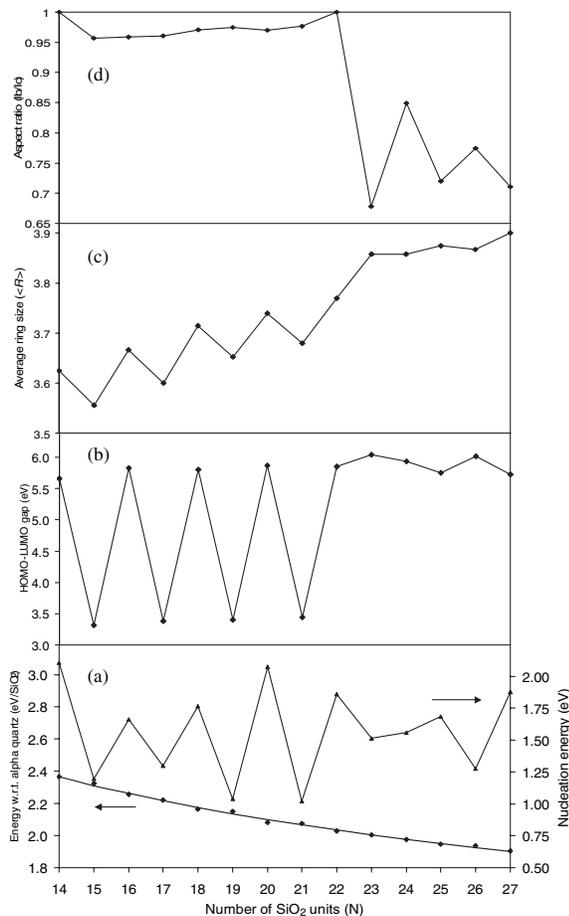
FIG. 2. For  $(\text{SiO}_2)_N$   $N = 14$ –27: (a) Cluster energies (eV/ $\text{SiO}_2$ ) with respect to the bulk extrapolated limit (left), nucleation energies (eV) (right). (b) HOMO-LUMO gap (eV). (c) Average  $(\text{SiO})_R$  ring size  $\langle R \rangle$ . (d) Aspect ratio ( $I_b/I_c$ ).
