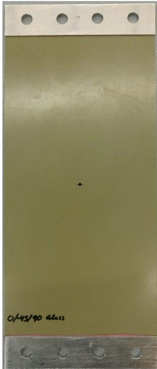
Figure 37: Prepared fatigue specimen
