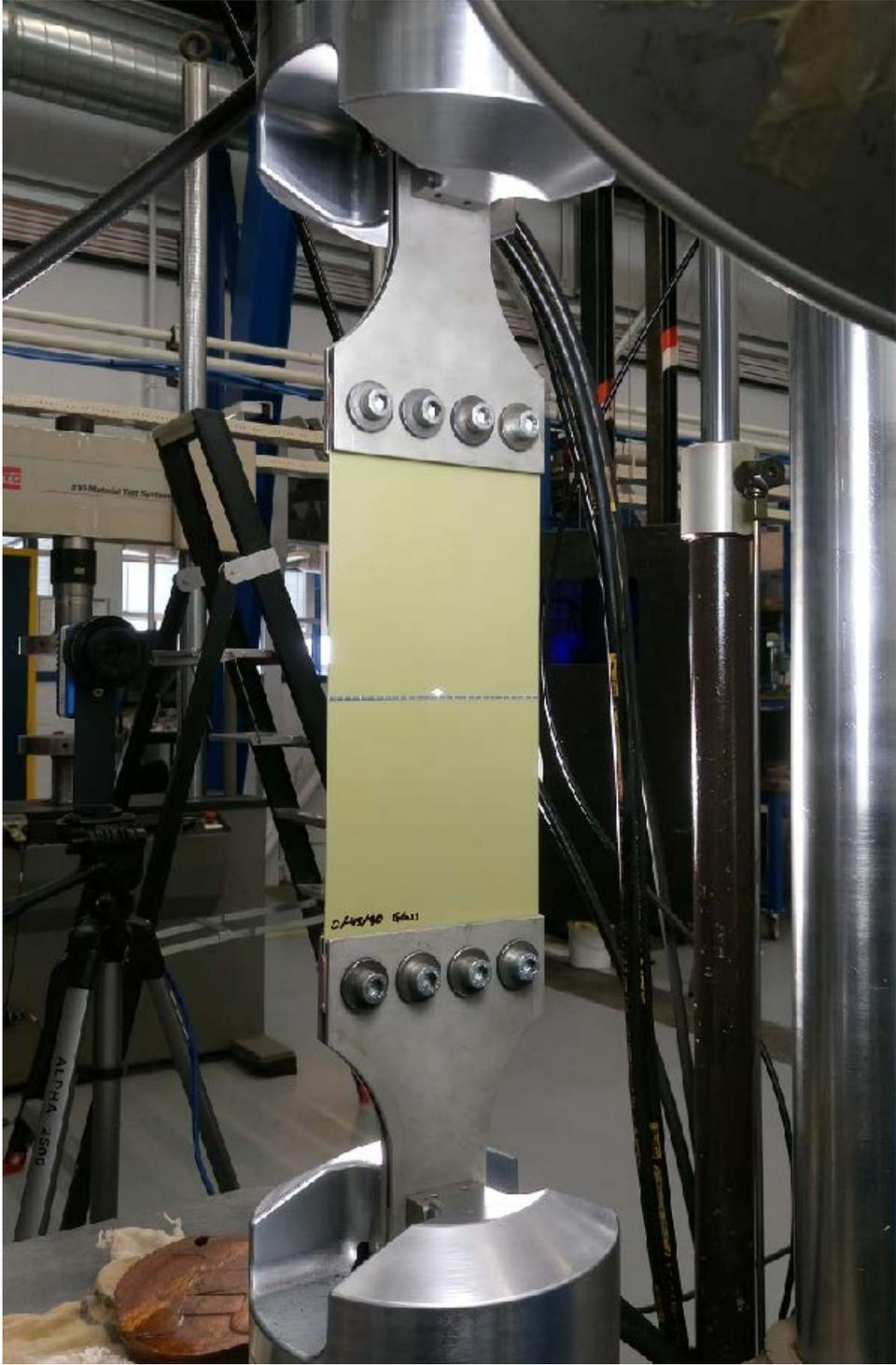
Figure 38: Fatigue specimen loaded in a Zwick 810 100kN fatigue machine.
