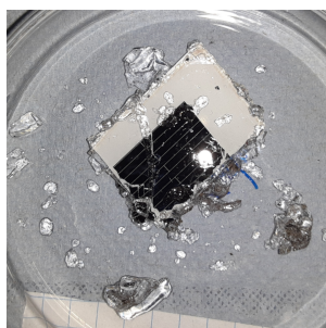
Figure 4.5: Result of xylene test, result shows major swelling of the sample.
