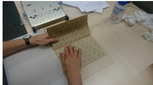
Figure G.2: Use your fingers to press the tape on the PMMA.
