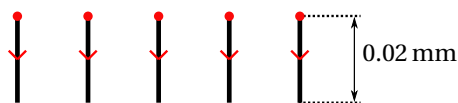
Figure G.19: Small 0.02 mm lines are drawn for generating the DXF. Because of the low frequency the laser only fires one pulse at the beginning of each line, at the location of the red dot. The result is a pattern with holes.
