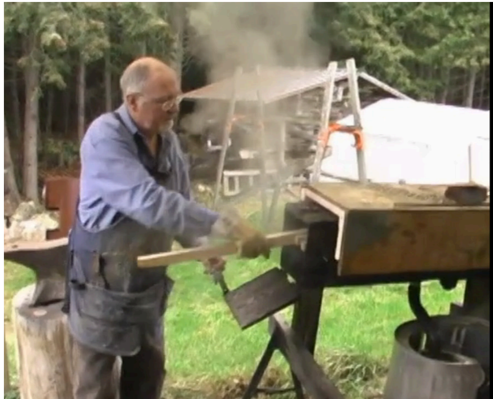
Steaming bamboo ref: www.bamboocraft.net
