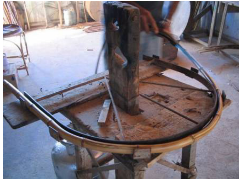
Bamboo bending form work ref: www.bamboocraft.net
