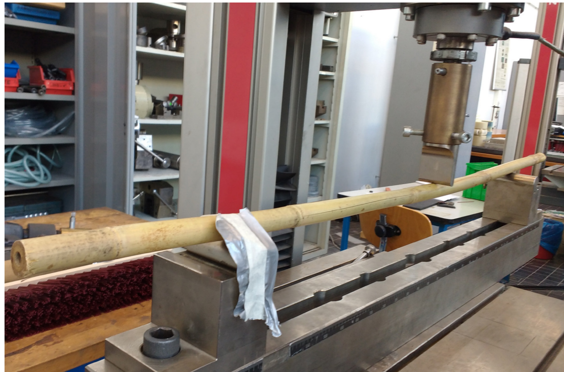
3-point bending test. Graph showing maximum deflection and yield limit.
