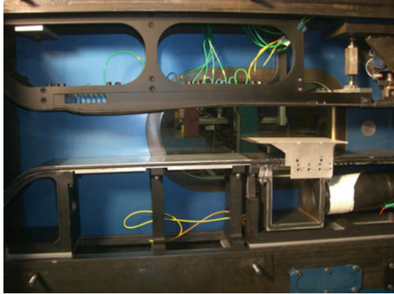
Fig. 1 Test set-up with the Mach 1.3 half nozzle in the S8Ch wind tunnel (w/o shock generator wedge)
