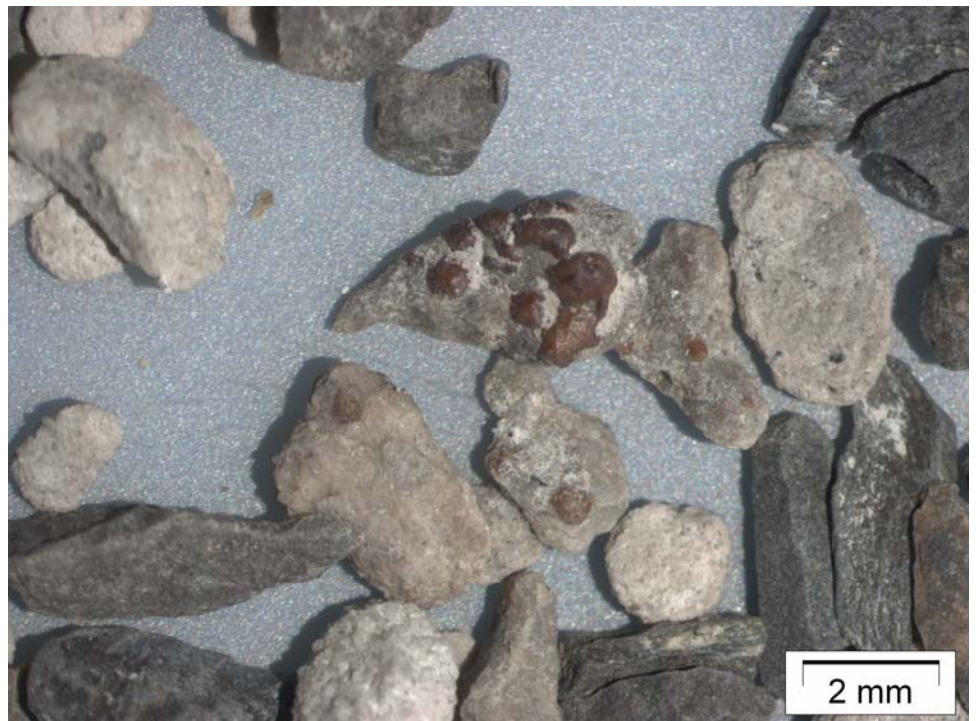
Figure 1806b Big siderite spherulites on sandstone cuttings
