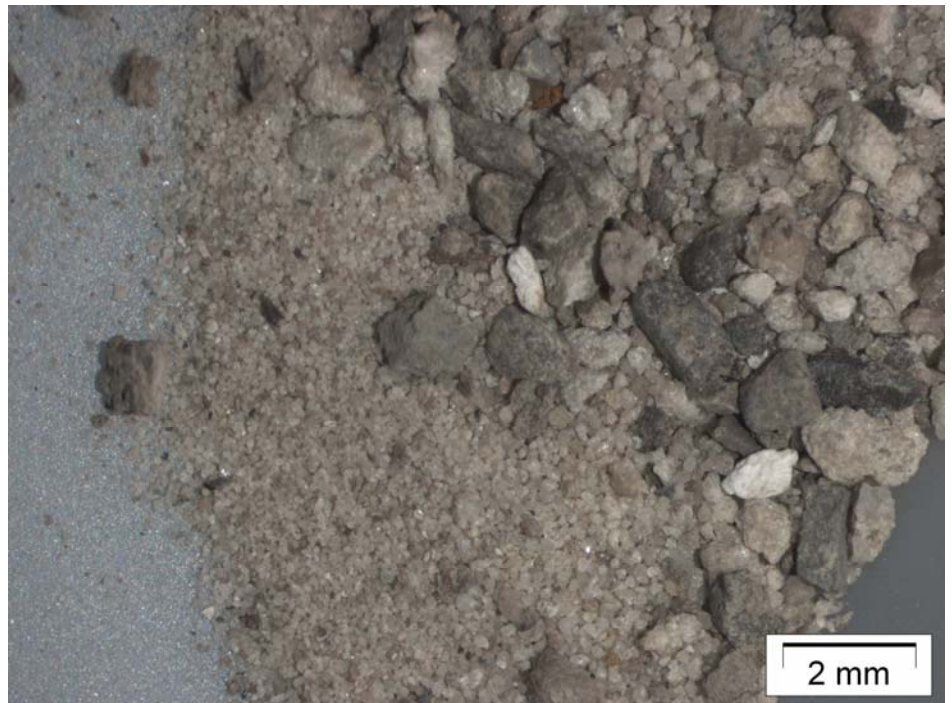
Figure 1840b Fraction < 1 mm with very small loose quartz grains
