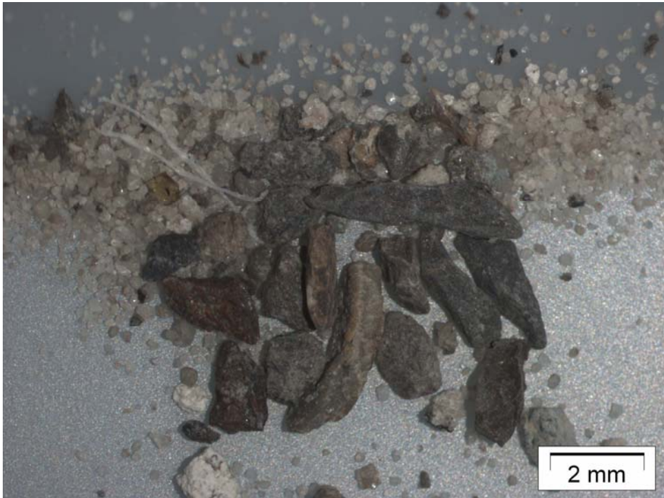
Figure 1798b < 1 mm fraction, containing a high amount of loose quartz grains and elongated claystone cuttings.
