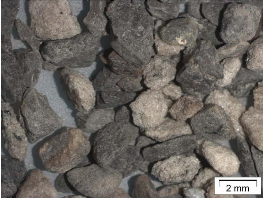
Figure 1798b < 1 mm fraction, containing a high amount of loose quartz grains and elongated claystone cuttings.
