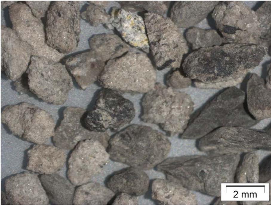
Figure 1850b Picture of the small fraction (< 1 mm) where you can see the amount of returns is quite low
