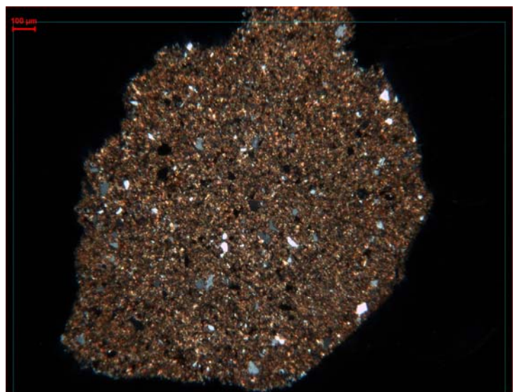
Figure 1918d; cutting no. 14 A photo of a siderite cutting with enabled analyzer.
