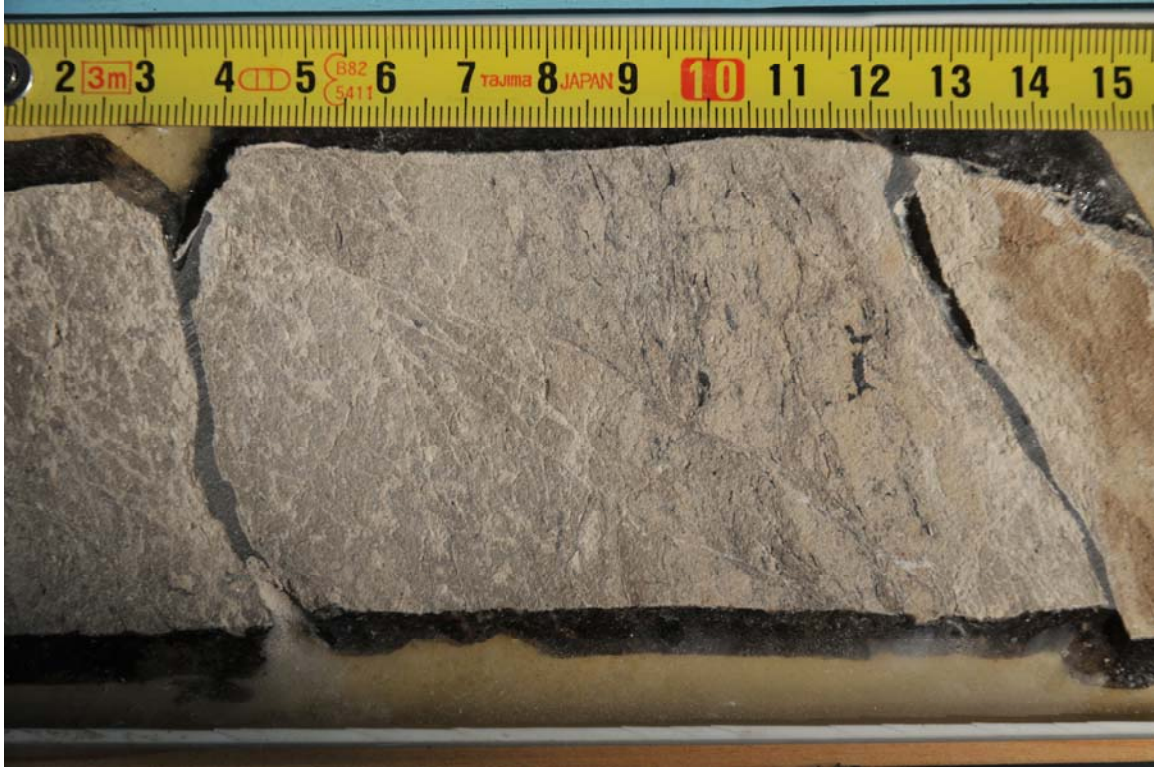
Depth: 909.8 – 910.3 m (Fractured dry)
