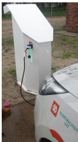
Fig. 5 V2G-DCAC unit connected to the FCEV.
