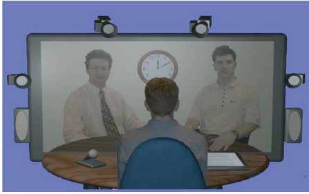
FIGURE 1: The mock-up of one VIRTUE station where the real table is extended seamlessly into the virtual table in display. The full-size remote participants are rendered as arbitrary 2D video objects and their synthesized looks will change in line with the local participant's head position. The two cameras mounted on the left and top-left side of the screen provide two video streams for 3D analysis and view synthesis for the left viewer in the display; likewise for the two right-hand side cameras. The eye-to-eye contact, normal habitual hand gesturing, and gaze awareness are expected to be maintained.
