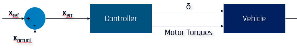
Figure 5.1: Block diagram of vehicle model and controller. "x" is a state vector consisting of yaw rate, sideslip and longitudinal velocity
