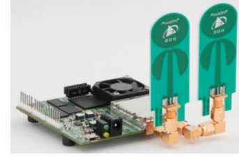
Fig. 3. A single Humatics PulsON P410 sensor with antennae, as used in the distributed networks in both case studies.
