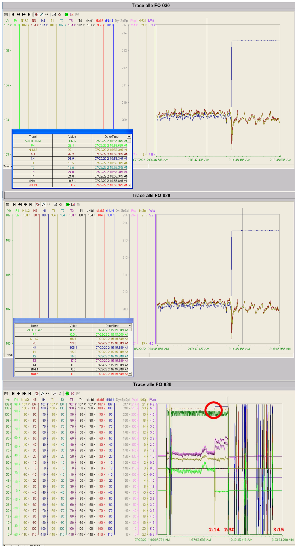
Figure 6.21: Top and middle pictures show a close-up of the rpm values of the four drive units with respective values before and after the event. Bottom picture is an overview with time notations
