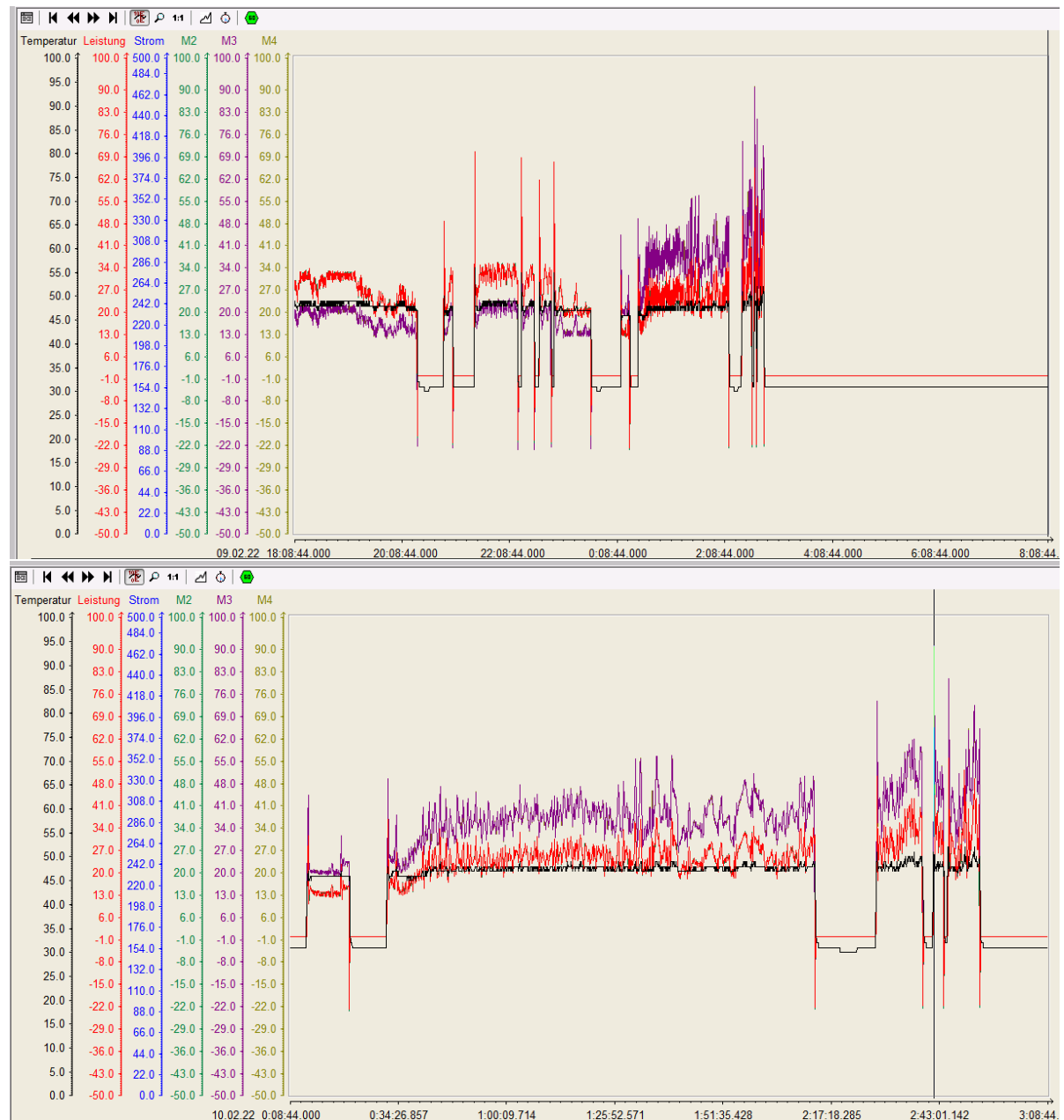
Figure D.2: Operation of belt 240 on the day of the event (10 February 2022). As can be seen there is an increase in scattering and values of power output of all drive units
