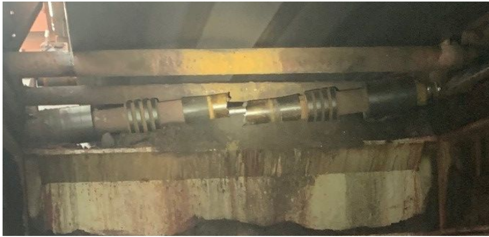
Figure 6.2: Broken Stutzringroll on belt 010 (6 July 2022) [16]
