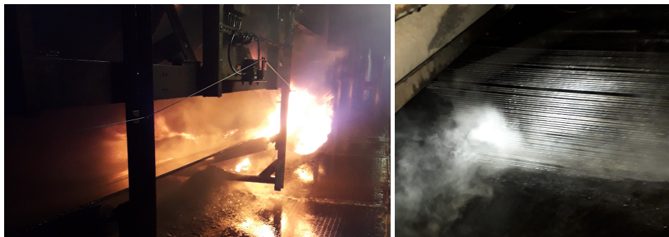
Figure 6.7: Pictures of the fire in belt 171: Left picture with fire, right picture shows the steel cords after extinguishing (rubber melted). Both pictures taken on 31 January 2022 [16]
