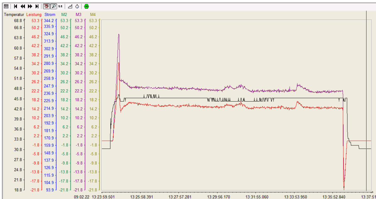
Figure D.1: Regular start-up and stopping of a conveyor belt system. Traces are from belt 240 on 9 February 2022
