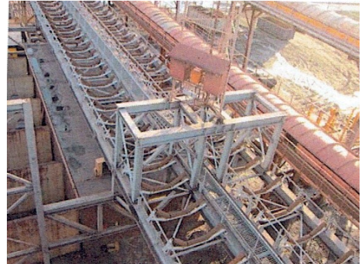
Figure 1.14: The frame and idlers shown without the belt (page 18 [67])
