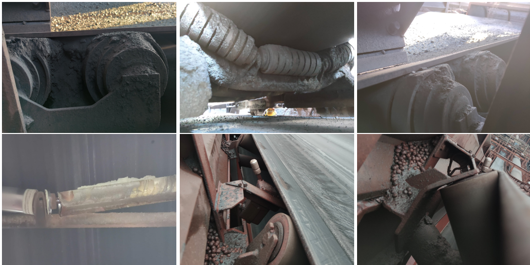
Figure 6.3: Examples of contamination in idlers: Top three pictures taken on 22 Nov 2021, bottom three pictures taken on 16 Feb 2022 [16]
