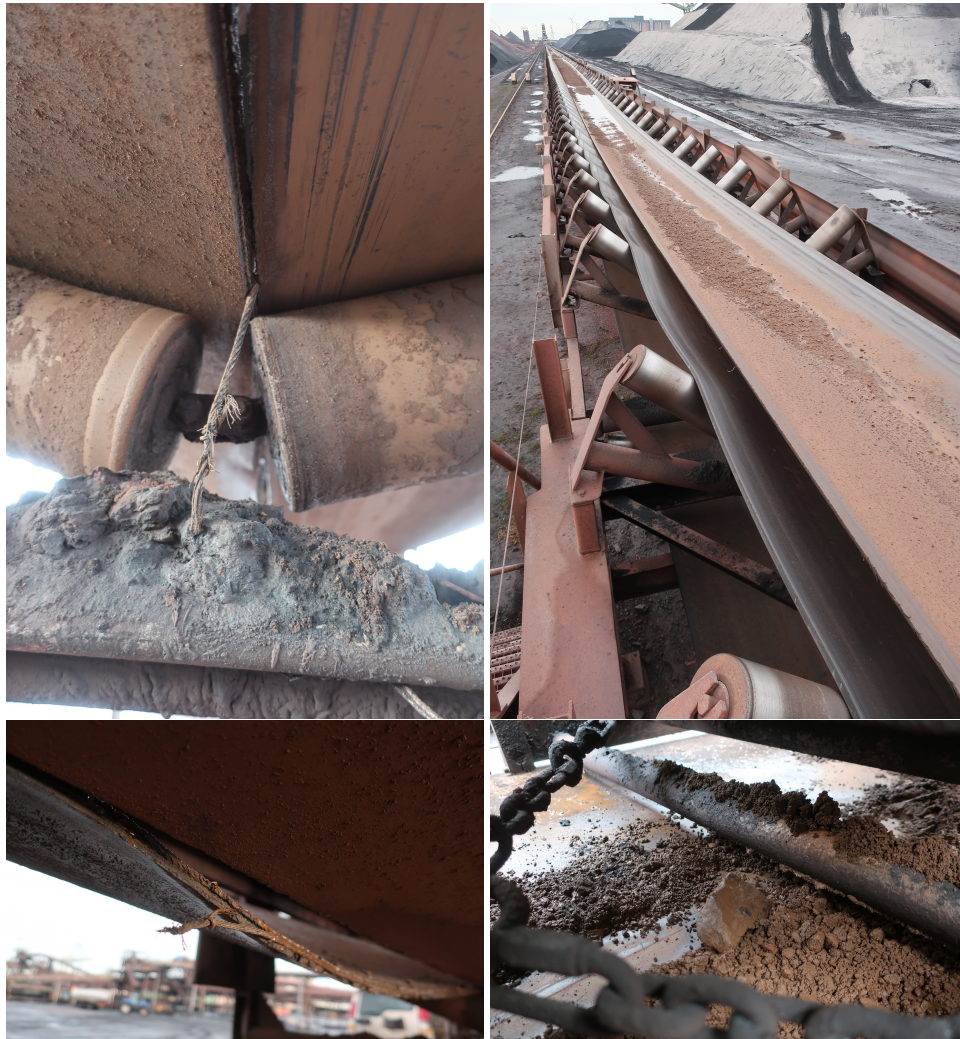
Figure 6.11: Tear in the belt 240, pictures taken on 10 Feb 2022 [16]. Top and bottom left: close-up of tear, where steel cord came loose. Top right: belt split in half, halves lay on top of each other. Bottom right: spillage and build-up material, larger rock which came along with the load
