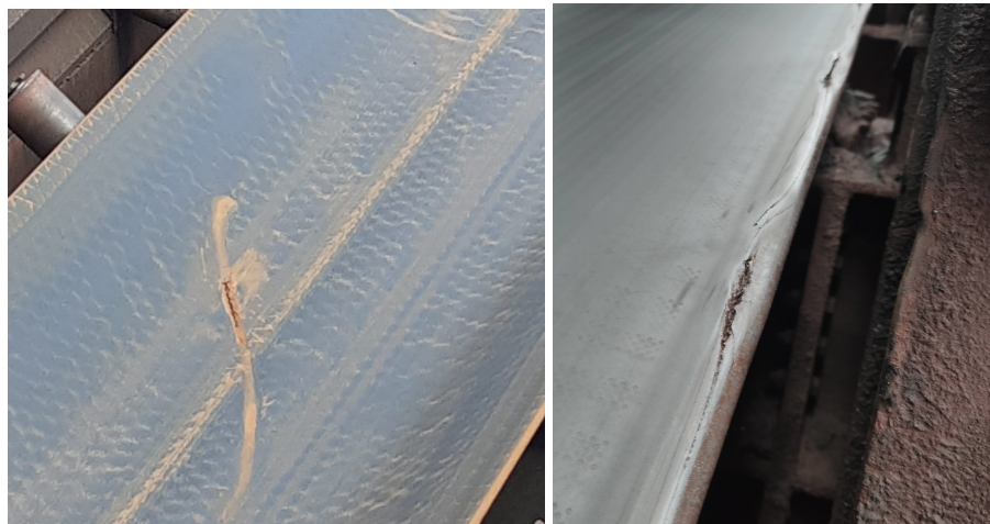
Figure 5.6: Belt damage: a tear and dent in belt 020 and a tear on the edge of the belt (16 Feb 2022) [16]
