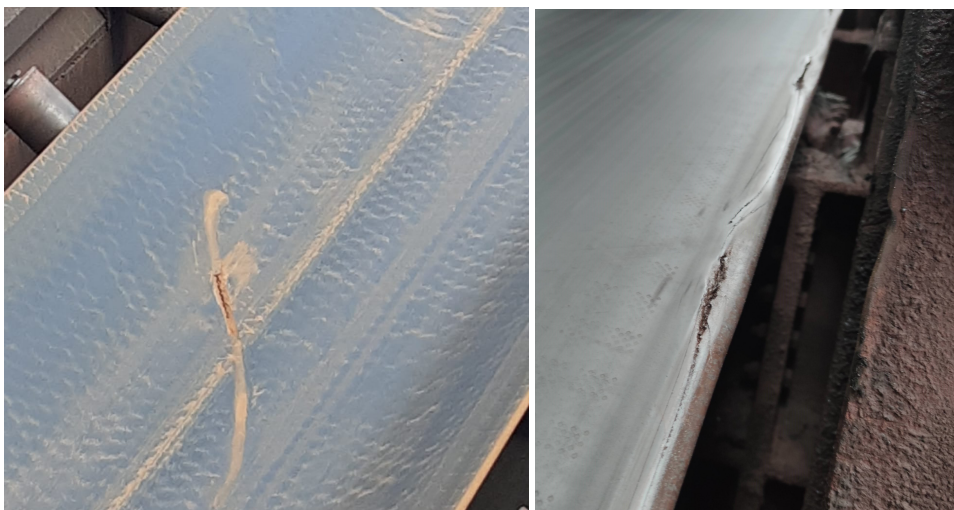
Figure 6.1: Belt damage: a tear and dent in belt 020 and a tear on the edge of the belt (16 Feb 2022) [16]
