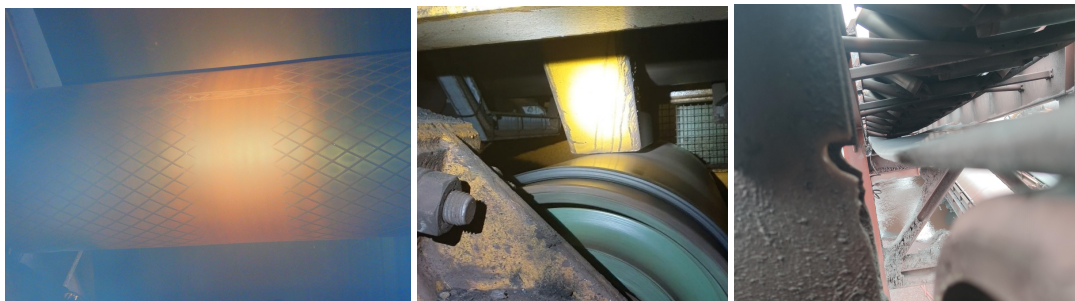
Figure 6.4: Examples from wear. Left picture shows a drum which is worn out in the middle part and became smooth. The remaining profile on the edges of the drum are still visible. Middle picture shows a piece of metal that runs into the belt, creating damage to the rubber (9 February 2022). The right picture shows a worn out structure where the returning belt has continuously run into the structure (16 February 2022)
