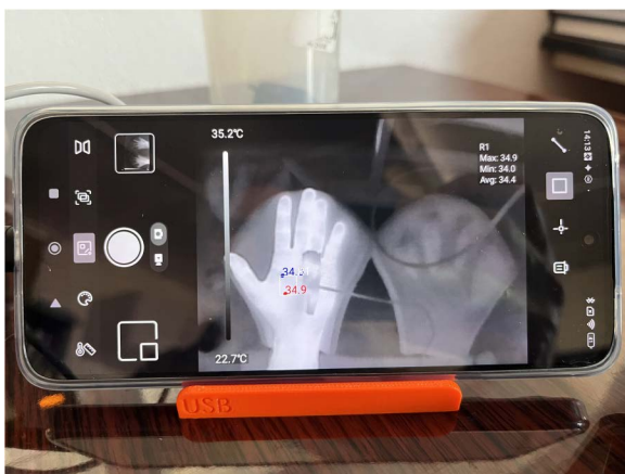
Fig 5. The phone screen during the accuracy test, showing the rectangle for reading the average temperature that is displayed in the top right corner.
