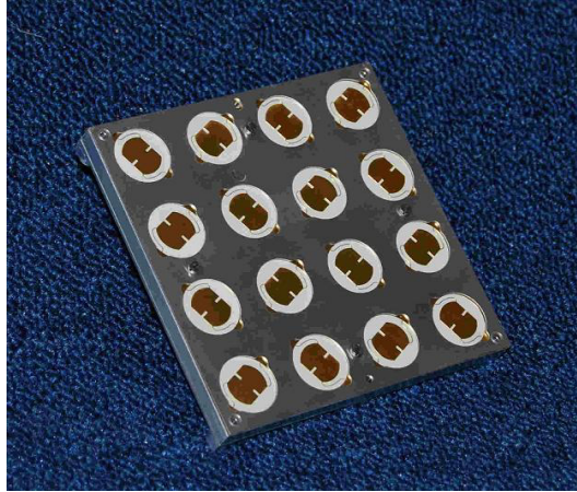
Figure 5.2: Completely assembled tile. The 16 parasitic patches are visible.
