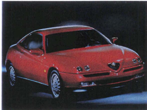
Figure 2.1: Alfa Romeo GTV Coupe hood, a typical SMC product
