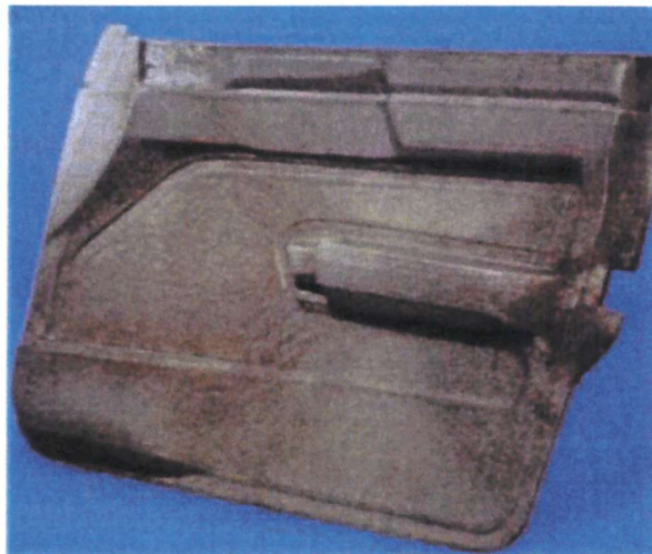
Figure 2.13: NFRP indoor panel
