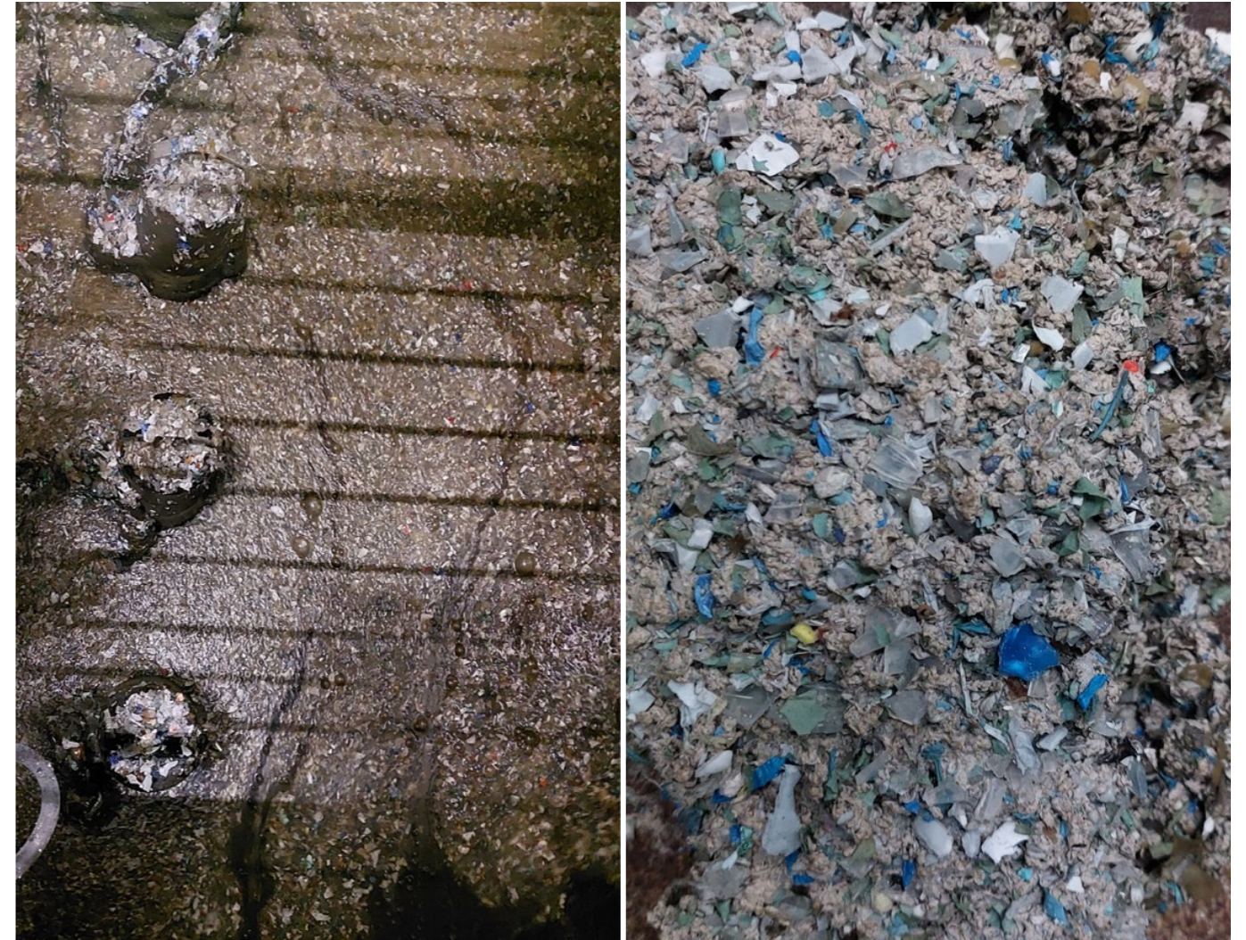
Figure 64: Solid waste mixed with wastewater before sterilization (left) and after sterilization (right)
