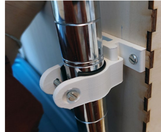
Figure 35: : The attachment during removal (sliding upwards)
