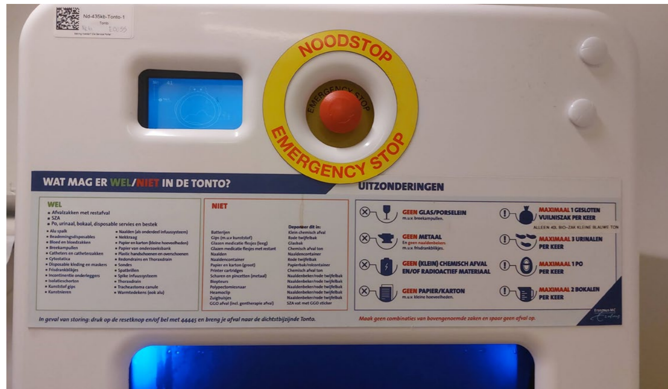
Figure 105. The rules about what can go into the Tonto, what cannot and maximum amounts.
