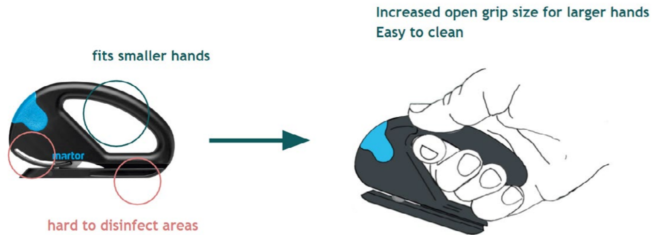
Figure 32: Redesign of the cutter to fit the ICU context.
