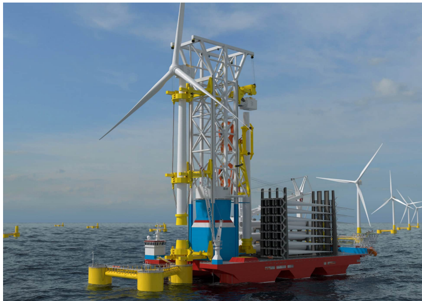
Figure 1.2: Render showing the Huisman Windfarm Installation Vessel concept, pictured installing a wind turbine on a semi-submersible floating support structure
