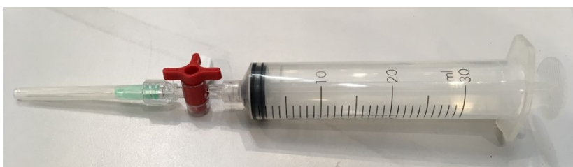
Figure 4.6: Syringe with Luer Lok connection to take a gas sample of the VLE inside the stripping column.
