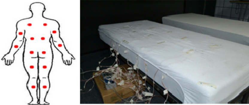
Fig. 6.2: Location of RTDs on the mattress pad material (on the left, under the thin cover) and their corresponding position on the subject's skin (red points)
