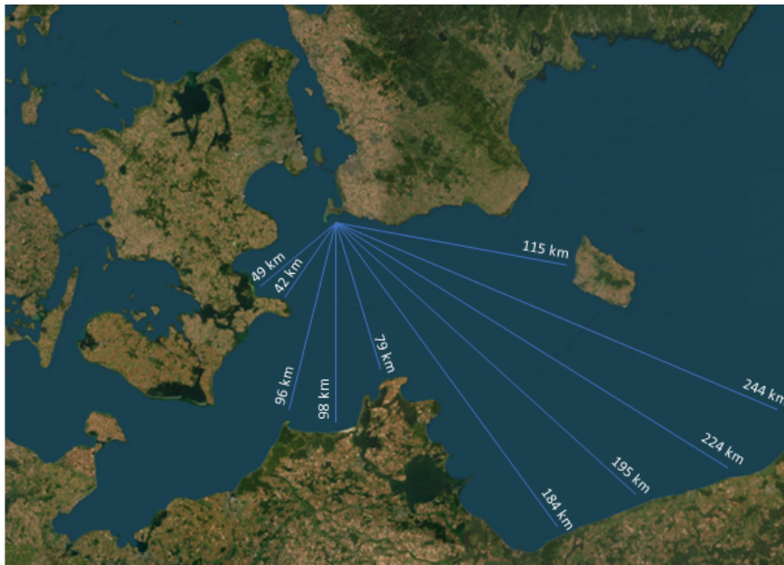
Figure 5.7: Fetch length to the study area, measured in various angles in Google Maps.
