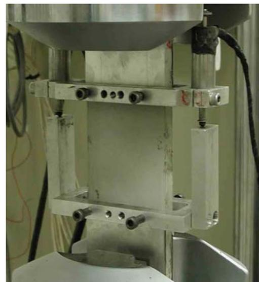
Figure 2. Setup for uniaxial tensile test.
