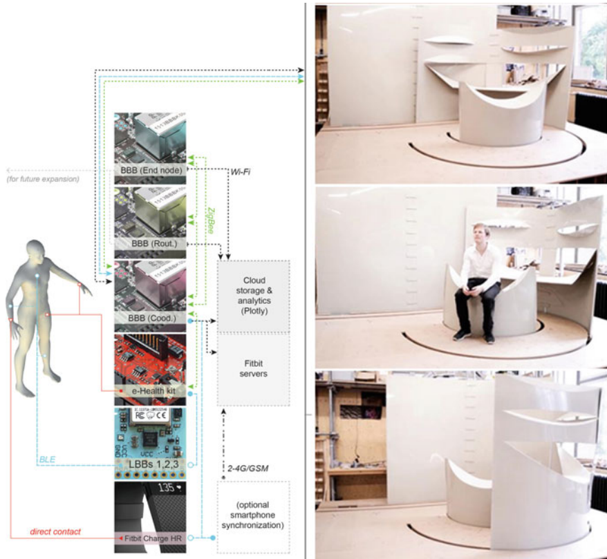
Fig. 5.1 Design-to-Robotic-Operation (D2RO) links computational mechanisms and services to spatial reconfiguration for the promotion of occupant well-being (Liu Cheng and Beir 2016a, b). Left: Basic form of the System Architecture, illustrating the relationship between (1) the Local System, (2) the Wearables Subsystem, and (3) the Cloud/Remote Services Subsystem, which are conceived as the essential features of D2RO. Right: Proof-of-concept prototype whose physical transformations actuate in response to sensed and processed data
