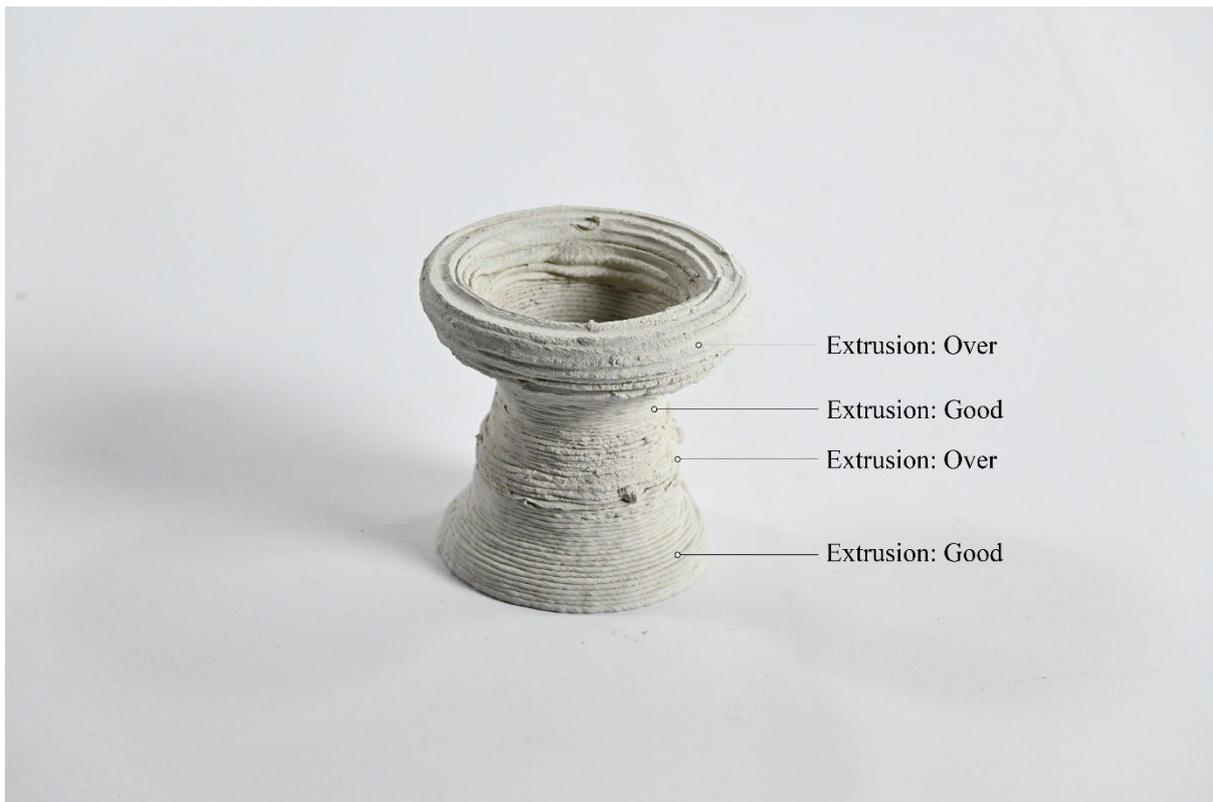
Figure 2.4: clay extrusion changes in one prototype printing due to slight clay mixture changes
