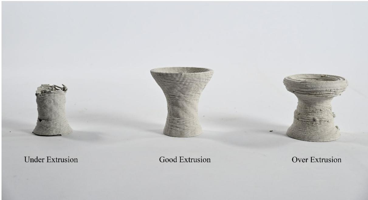
Figure 1.5: Extrusion label categories demonstration according to general quality (elevation view)
