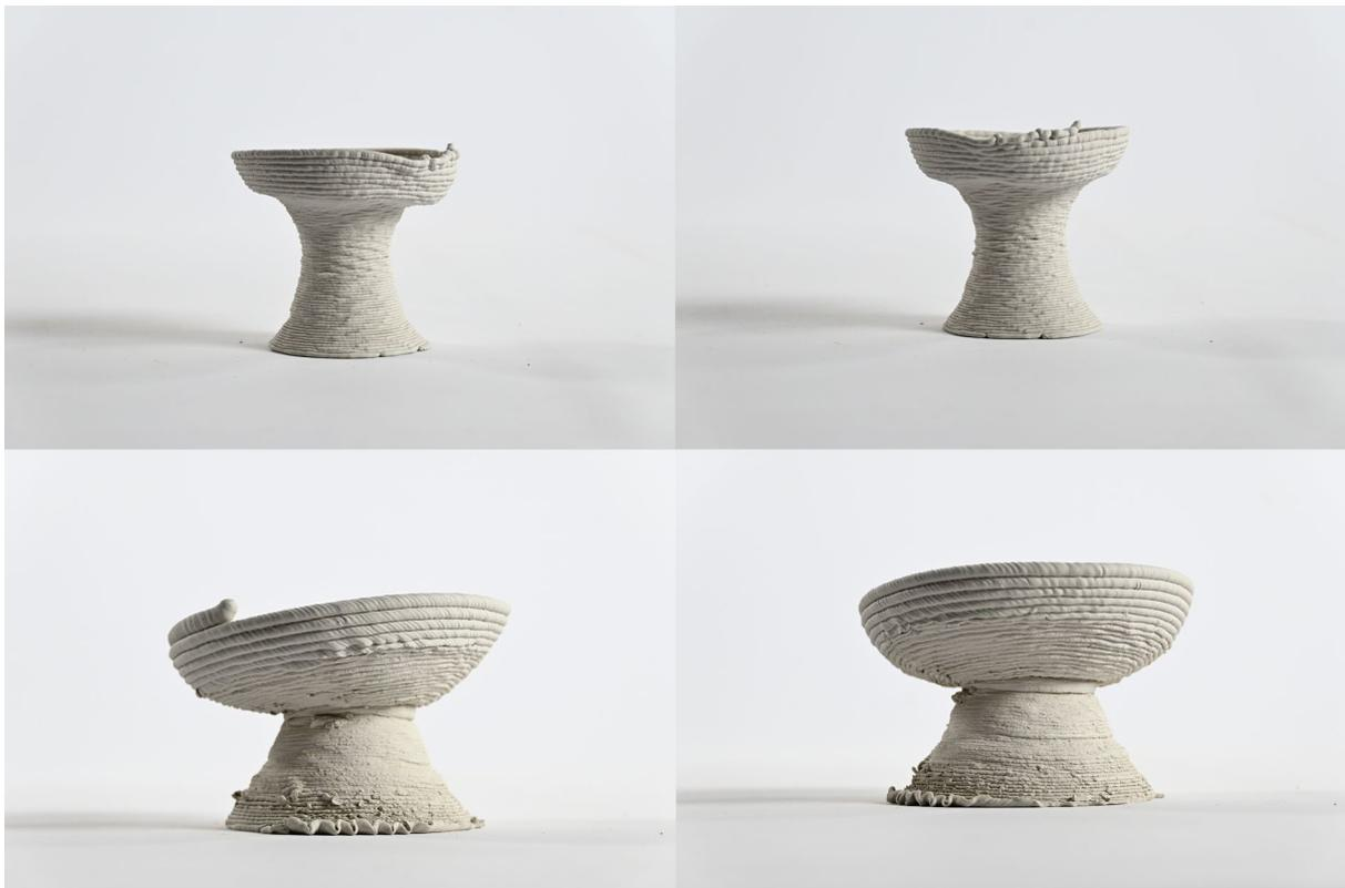
Figure 2.37: Examples of overhang sagging without collapse
