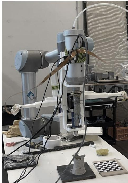
Figure 1.2: Experiment setting of 3DCP.
