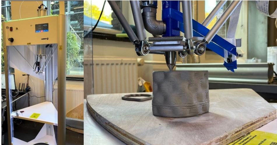
Figure 2.6: WASP 40100 Delta printer (left) & printing set up (right)
