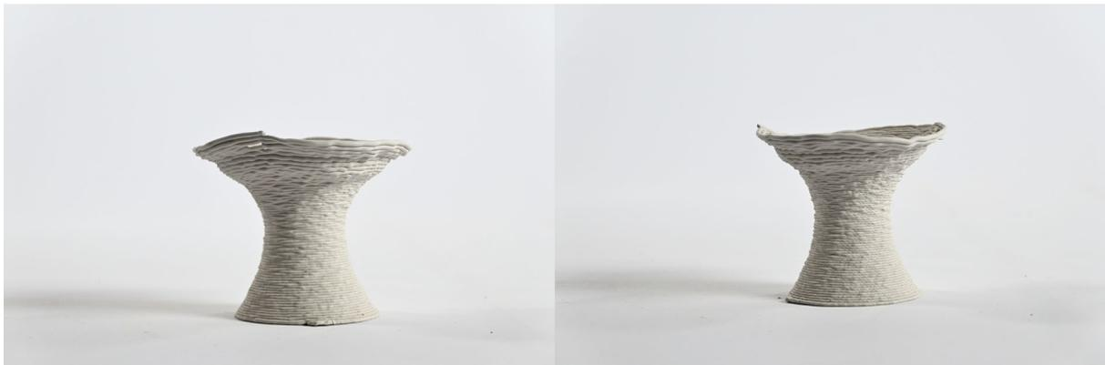
Figure 2.36: Example of overhang part under-extrusion
