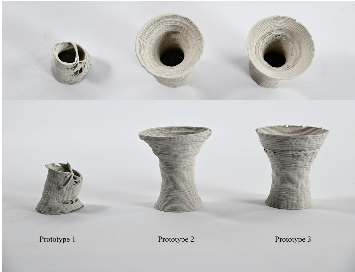
Figure 3.2: Comparison of Default Printing (1,2) and Real-Time calibration printing (3)
