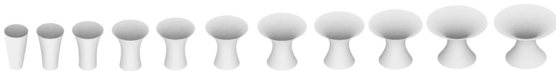
Figure 4.2: the dataset intended to be printed with different inclined angle of overhang
