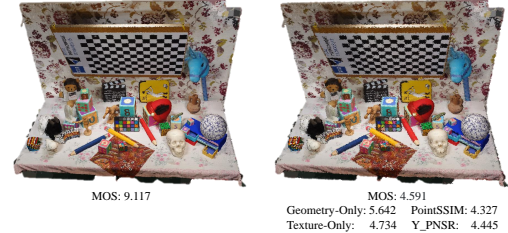
Figure 3: Point cloud Unicorn comparison between learning-based and traditional FR metrics. The left side shows the reference Unicorn, while the right side displays the distorted version with geometry Gaussian noise (points randomly shifted within 0.02%).
